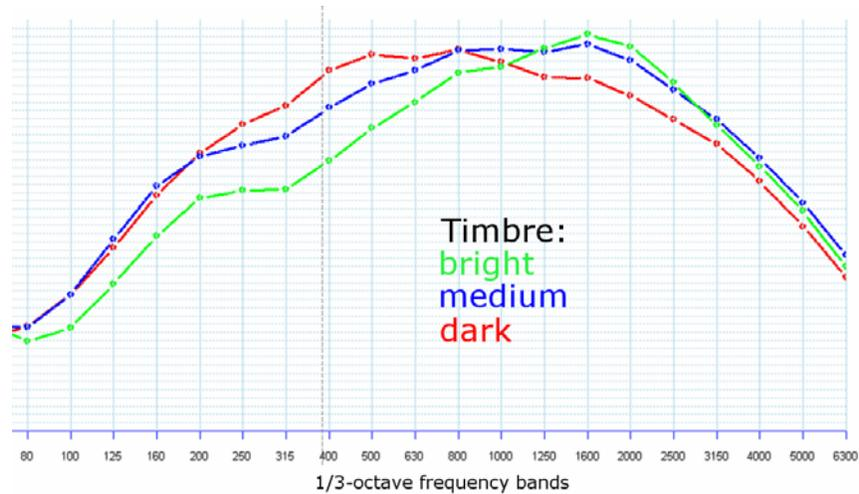
Figure 5. Mean value of the relative 1/3-octave levels in 21 frequency bands according to cluster membership
