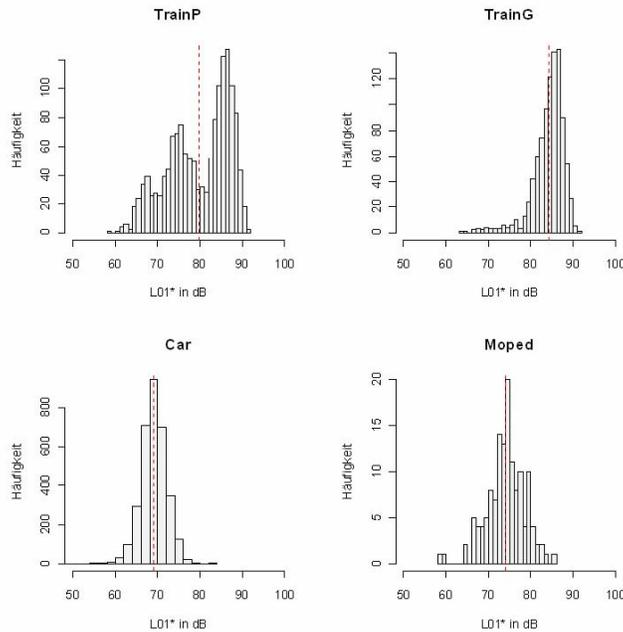
Figure 3. Period histograms showing the typical level distribution in L01\* dB(A): The bimodal distribution for passenger trains results from the combination of quickly passing trains and more slowly moving ones starting out [3][5].
