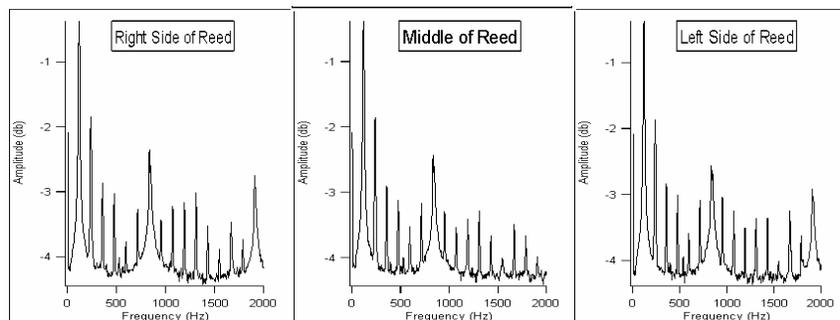
Figure 10.- Spectra showing the presence of the first torsional mode
