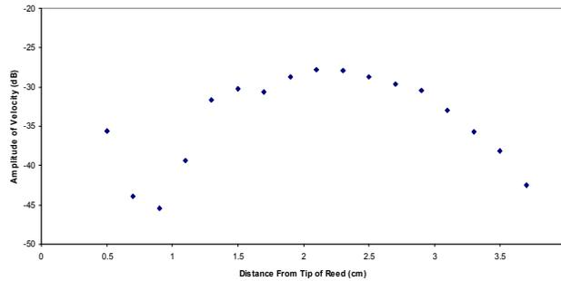
Figure 9.- Amplitude of the 805 Hz peak as a function of distance from the reed tip
