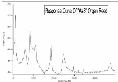
Figure 7.- A response curve for an organ reed showing several modes of vibration.
