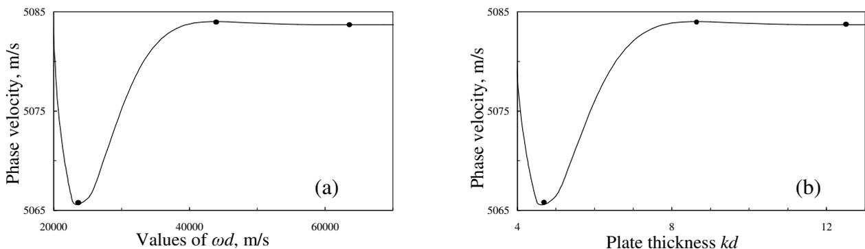
**Figure 2.** The non-dispersive Zakharenko waves representing extreme points of the phase velocity  $V_{ph}(\omega d)$  (a) and  $V_{ph}(kd)$  (b) shown by the big points for a fundamental mode of Lamb type waves ([110] propagation direction for Si).
