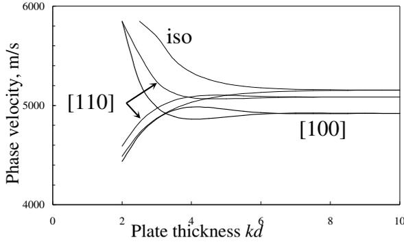
**Figure 1.** The phase velocity  $V_{ph}(kd)$  for fundamental modes of Lamb (type) waves.
