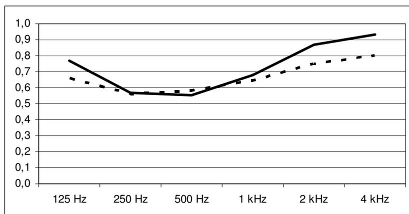
Figure 7. – Measured RT of above shown classroom without (—) and with (---) slats
