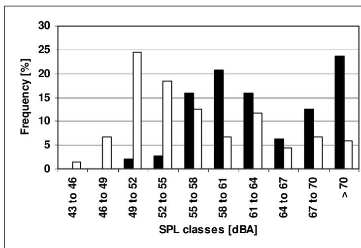
Figure 2. – Overall frequency distribution of the working SPL before (●) and after (○) refurbishment (school 1; incl. all observed lessons)
