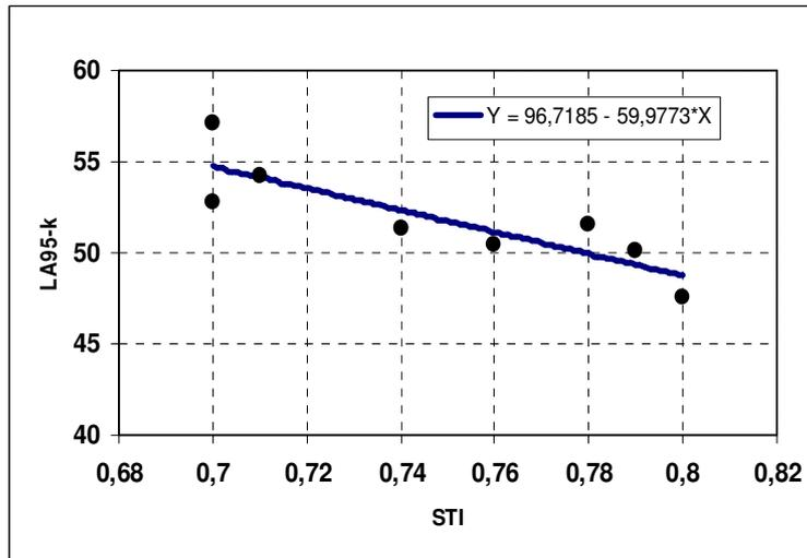
Figure 3. – Basic SPL in relation to the STI found for the 8 classrooms of school 2 with different acoustic properties; ground floor (●) and top floor (○)
