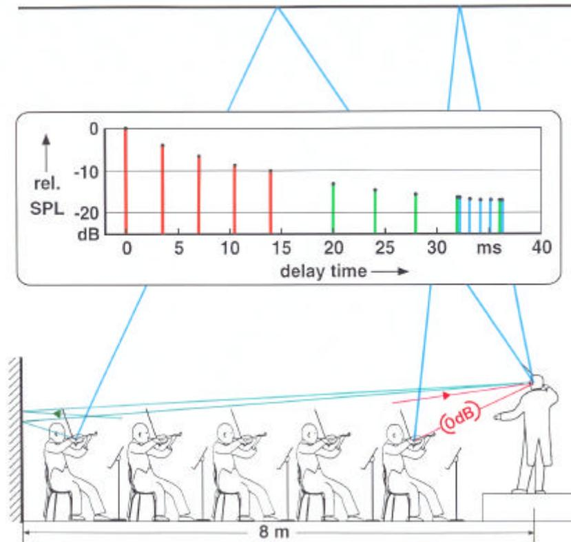
Figure 2.- Effect of a wall and a ceiling reflection on the sound field at the conductor's location
