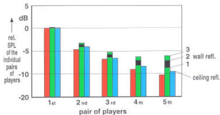
Figure 3.- Increase of the SPL at the conductor's location caused by wall and ceiling reflections
