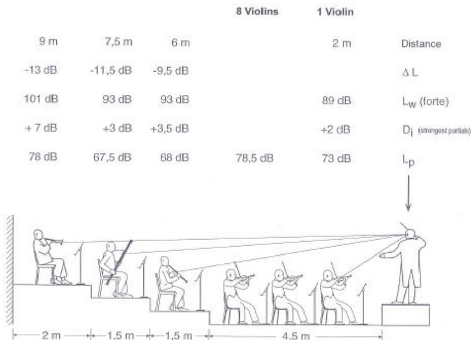
Figure 4.- Sound pressure level  $L_p$  of the direct sound at the conductor's ears derived from distance and related level attenuation  $\Delta L$ , sound power level  $L_w$  and directivity index  $D_i$
