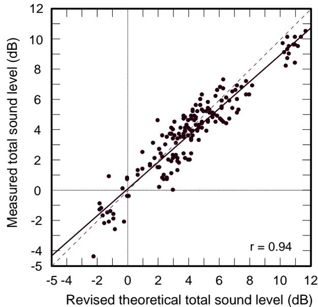
Figure 3. Measured vs. revised theoretical total sound level at mid-frequencies. 174 positions in 17 concert halls.
