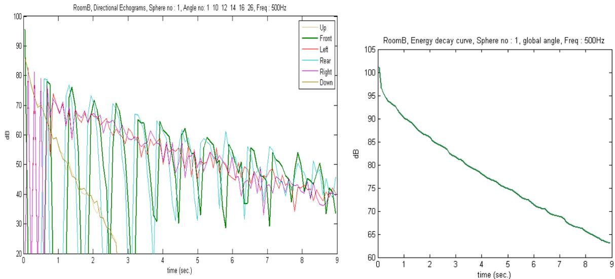
Figure 4.-Left : Directional echograms computed in Room B (500 Hz), for six particular directions of incidence. All reflections are specular ( $d=0$ ).
