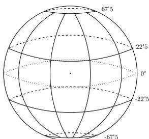
Figure 2.-Definition of the 26 solid angles around the listener's head (the azimuth discretization angle is 45 degrees).
