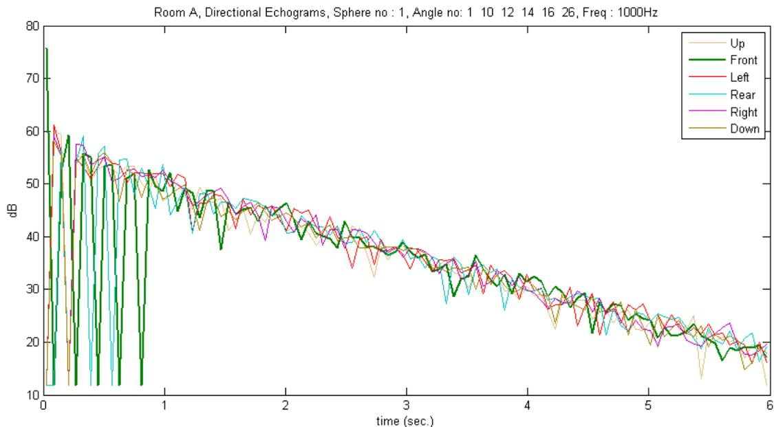
Figure 3.-Directional echograms computed in Room A (1 kHz), for six particular directions of incidence. All reflections are specular ( $d=0$ ).
