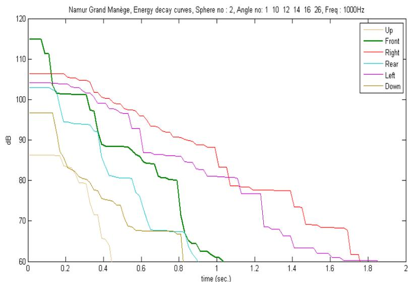
Figure 8.- Directional energy decay curves (1 kHz), computed in the concert hall with an acoustical treatment of the right wall (same receiver position as in figure 5).
