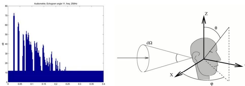
Figure 1.-A directional echogram gives the distribution of acoustical energy at the receiver (dB) contained in the solid angle  $d\Omega$ , versus time arrival (s).
