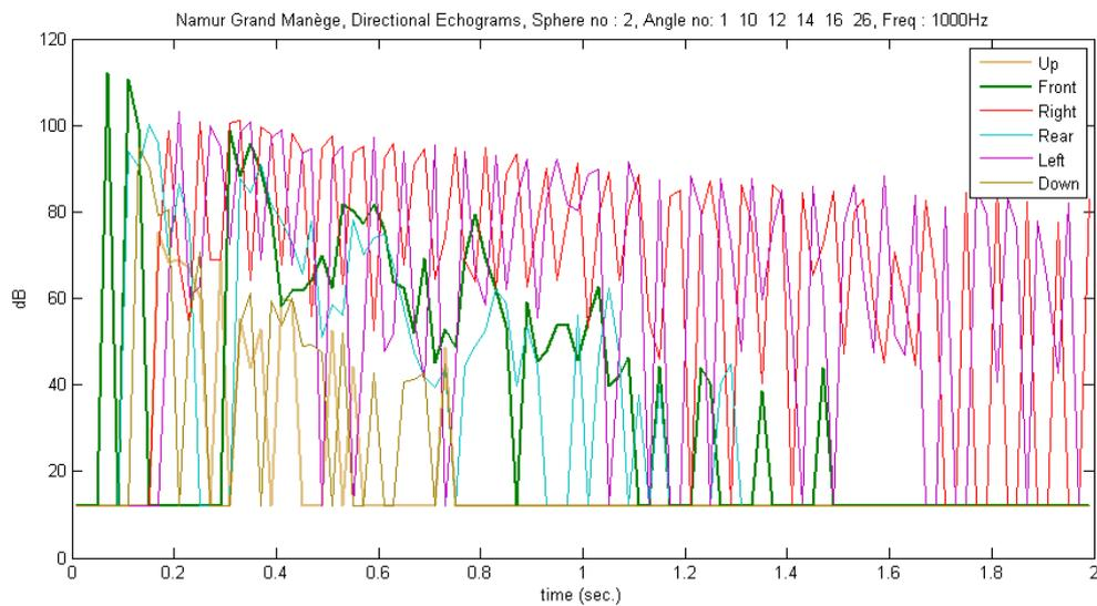
Figure 6.-Directional echograms computed in the concert hall (1 kHz), for six particular directions of incidence (same receiver position as in figure 5).
