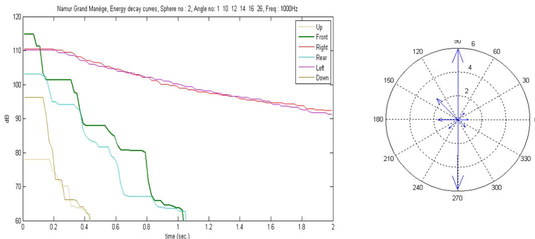
Figure 7.-Left : Directional energy decay curves (1 kHz), corresponding to figure 6. Right : Reverberation times T30 computed in the horizontal plane (0 degree is the “front” direction, 90 degree is the “left” one, ...).
