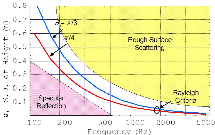
Fig. 3 Criteria of rough surface scattering.
