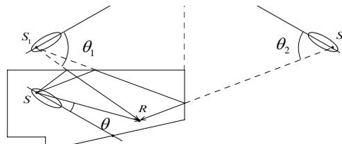
Figure 2.-Application of the source-directivity model to the image method
