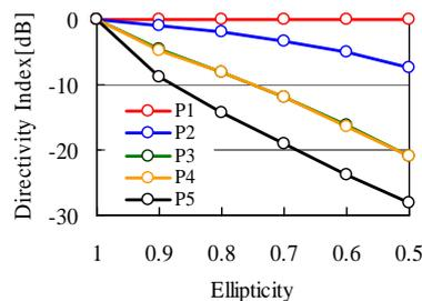
Figure 7.-Relation between the ellipticity and Directivity Index
