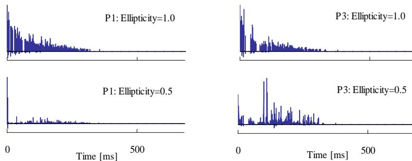
Figure 9.-Effects of source directivity on the impulse response
