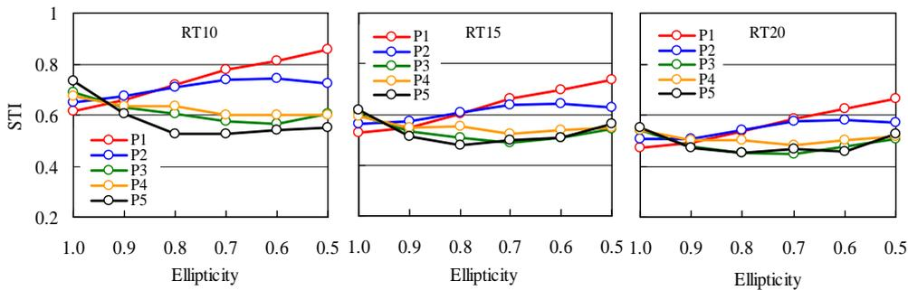
Figure 6.-Effects of difference in receiving point on STI
