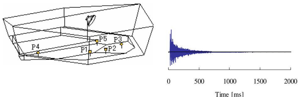
Figure 3.-A simple model of a hall, and an impulse response used in the calculation
