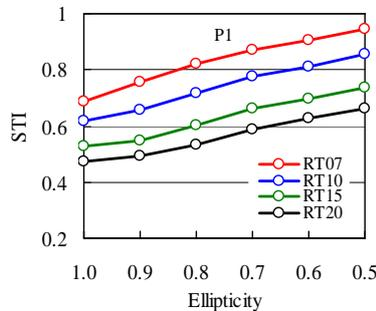
Figure 5.-STI variation at a point P1 with a parameter of the reverberation time
