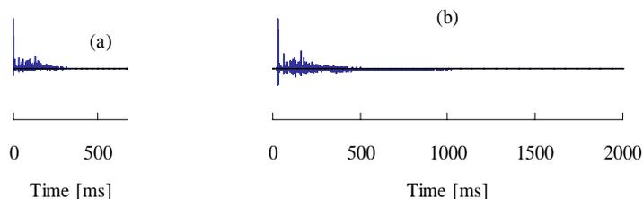
Figure 4.-Impulse response from the image method (a), and combined impulse response filtered at mid frequencies (b)
