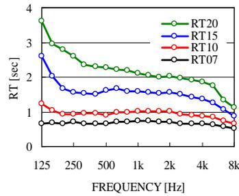
Figure 8.-Characteristics of the reverberation time used in the calculation
