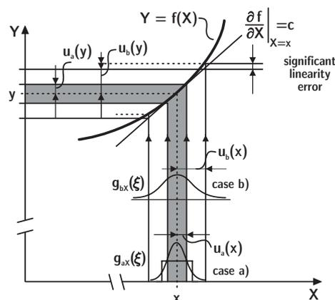
Figure 1.-Graphical representation [4] of the relationship between input- and output quantity.
