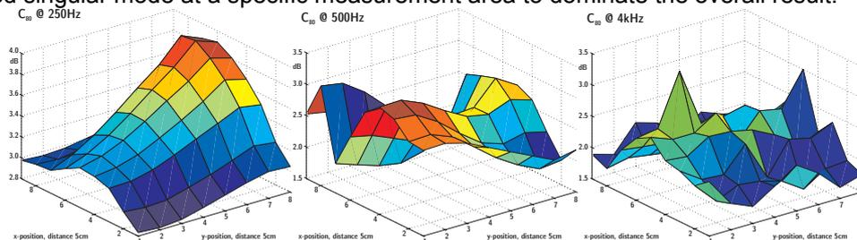
Figure 6.-Inner seat variation of  $C_{80}$  for 250 Hz, 1 kHz and 4 kHz octave bands
