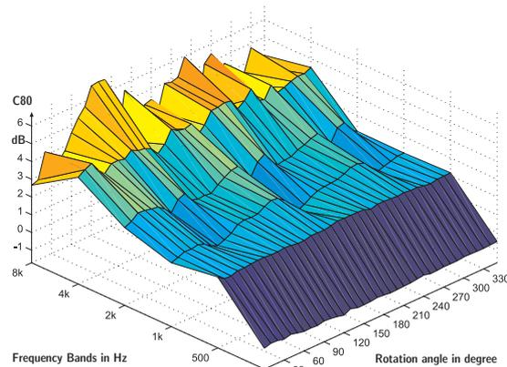
Figure 5.-Effect of the directivity of a sound source on  $C_{80}$  in a concert hall
