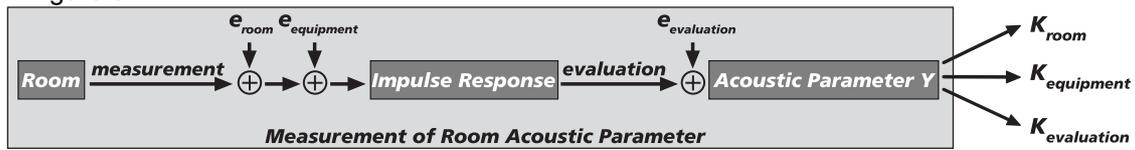
Figure 2.-Capsuled sources of measurement error
