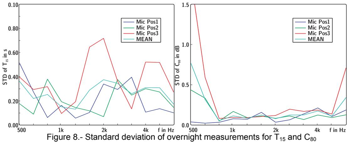
Figure 8.- Standard deviation of overnight measurements for  $T_{15}$  and  $C_{80}$
