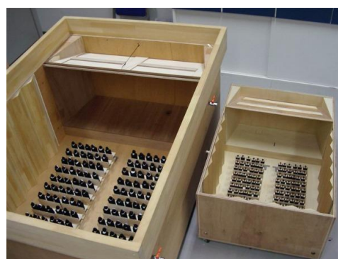
Fig.2. 1/10 scale model (left side) and 1/16 scale model (right side) simulating the same hall of 132 seats.
