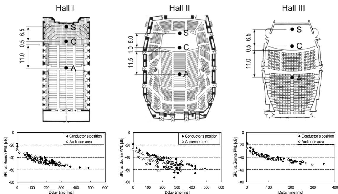
Figure 1.-Plans and reflect diagrams of 3 halls
