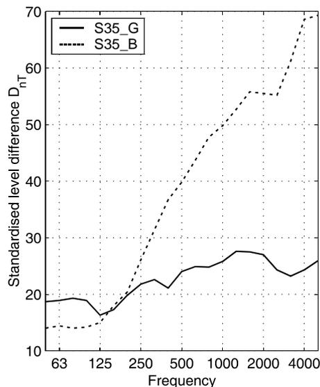
Figure 1.- Sound insulation curves of the two used conventional building situations used to auralise the two speech signals differing clearly in speech intelligibility. The standardised level difference  $D_{nT}$  illustrates the filtering of the original speech signal.
