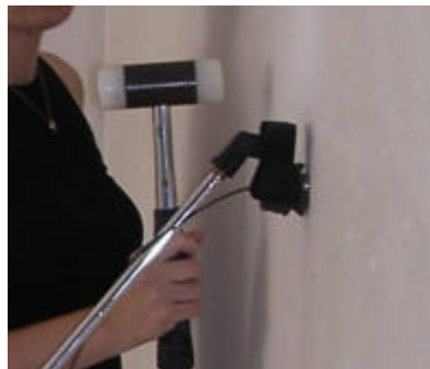
Figure 1. Hammer near accelerometer to measure the structural reverberation time
