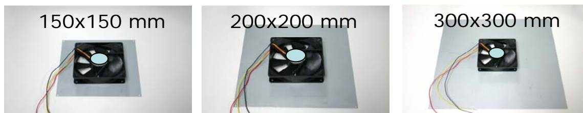
Figure 2. Steel plates and 92 mm fan configurations.
