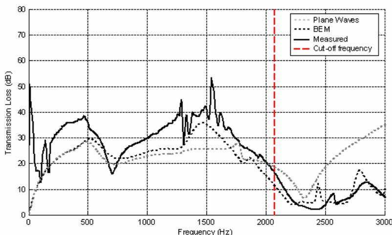
**Figure 8.** TL comparison for Configuration #5 : Plane Waves Method, BEM, measured
