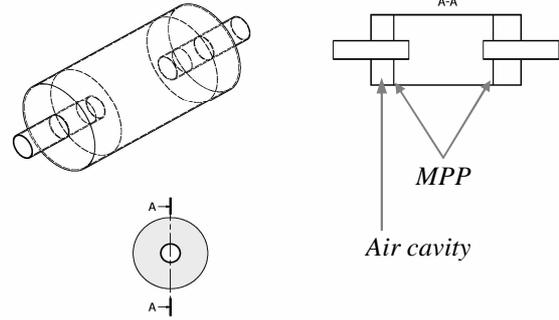
**Figure 2.** Muffler drafting
