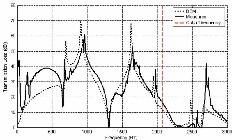
**Figure 5.** TL comparison for Configuration #2 : BEM, measured
