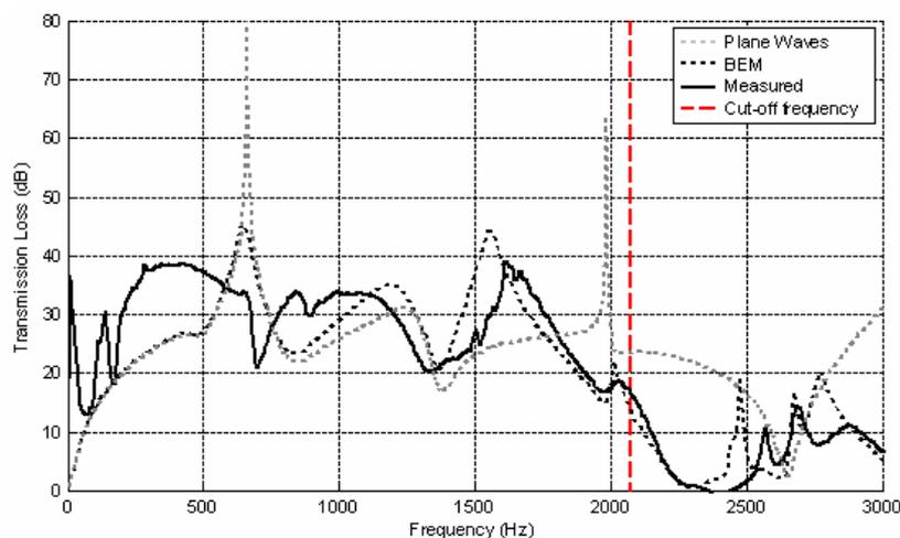
**Figure 6.** TL comparison for Configuration #3 : Plane Waves Method, BEM, measured
