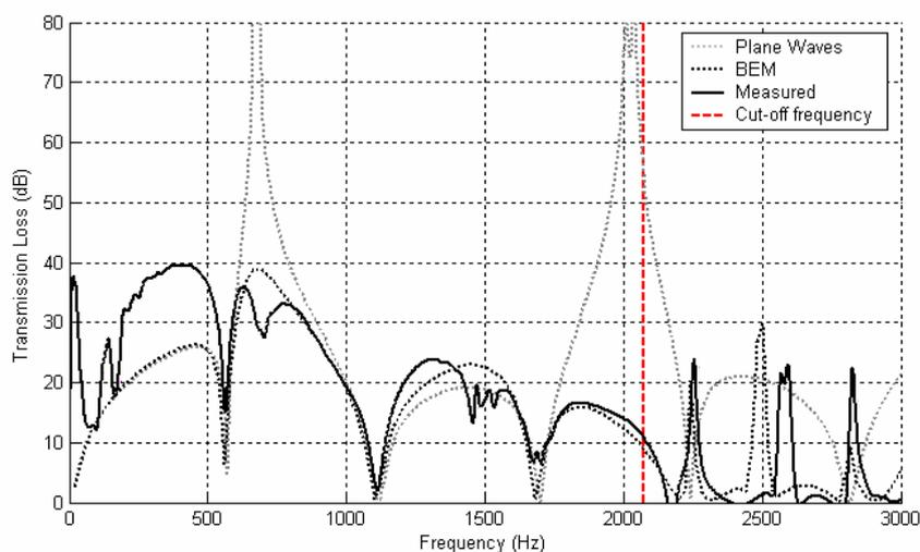
Figure 4. TL comparison for Configuration #1 : Plane Waves Method, BEM, measured
