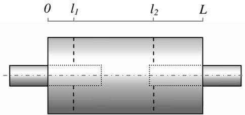
**Figure 1.** Muffler with extended inlet/outlet and MPP
