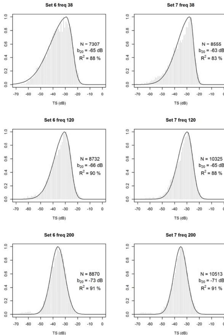
Figure 6. Observed (grey bars) against predicted (continuous line) TS distribution of the curve fitting procedure used to estimate  $b_{20}$  for each set and acoustic frequency.
