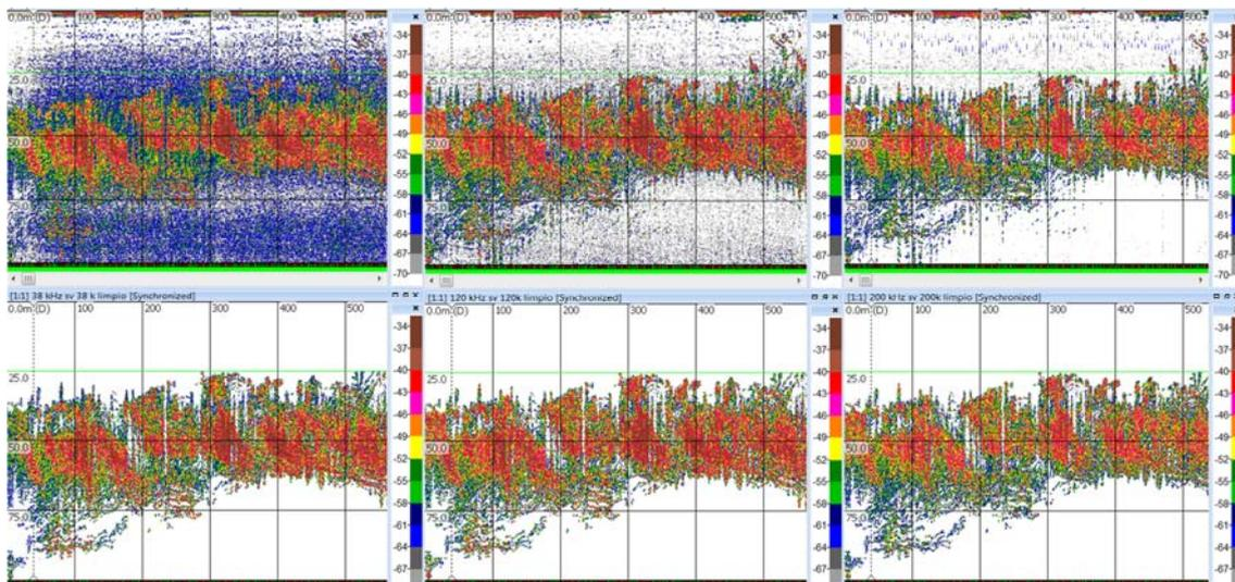
Figure 1. Sample echogram of set number 6 for the three frequencies, 38, 120 and 200 kHz from left to right. The upper panels show the raw echograms and the lower panels the echograms after the plankton / micronekton filtering.
