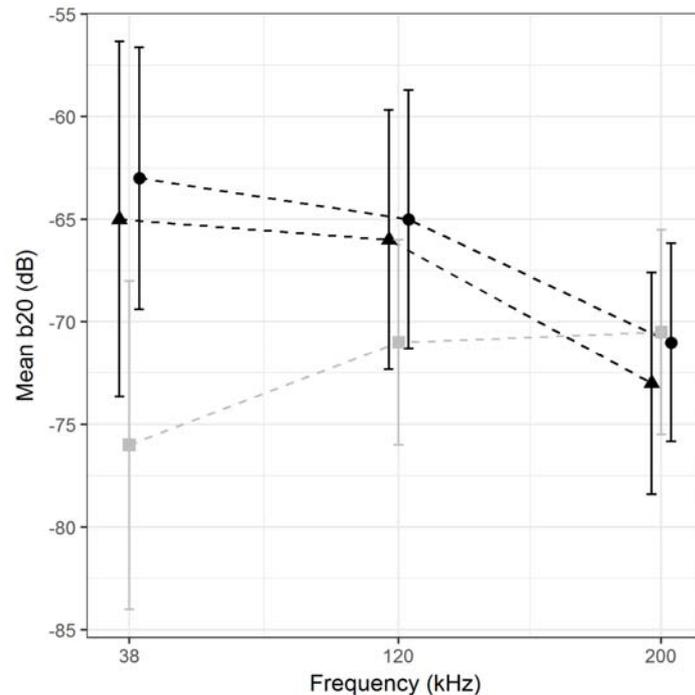
Figure 7. TS frequency response of bigeye tuna (black), triangles representing set 6 and circles set 7. In grey squares, TS frequency response of skipjack tuna, redrawn from Boyra *et al.* (2018). Error bars represent standard deviation.
