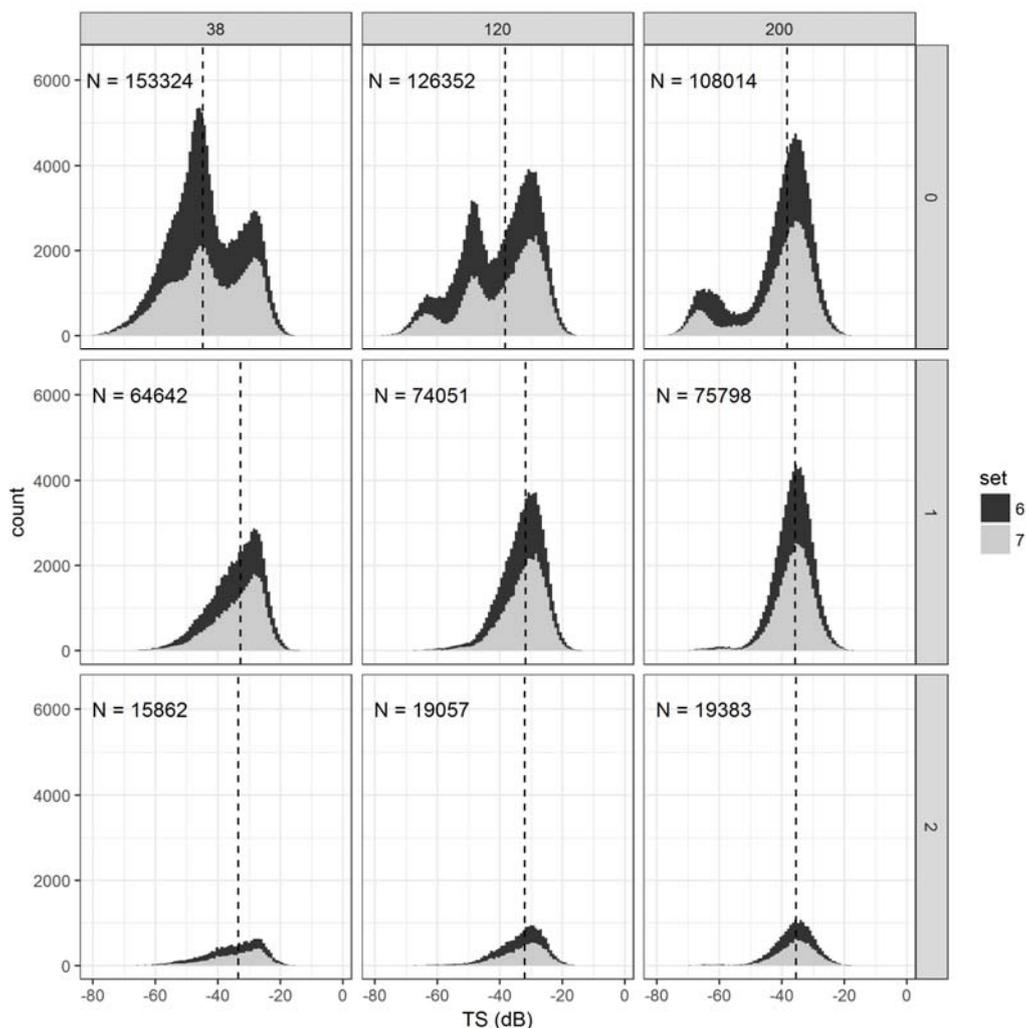
Figure 5. Histograms of TS values at the three frequencies for the incremental layers of filtering: (0) raw TS distribution without filtering; (1) filtered with the school masking; and (2) school masking plus multifrequency simultaneity requirement. Vertical dashed lines represent the median TS value and N is the remaining number of single targets in each step.
