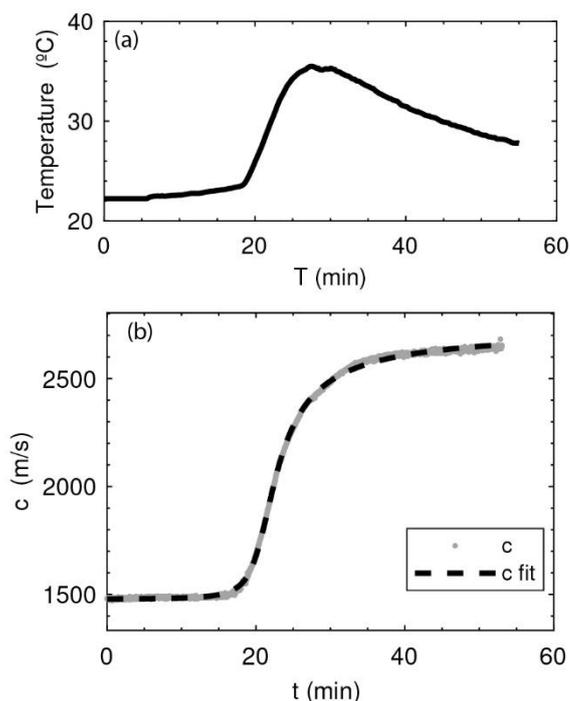
Figure 2. The temperature measured in the experiment in °C (a) and the speed of sound measured and close-fitting. (b)
