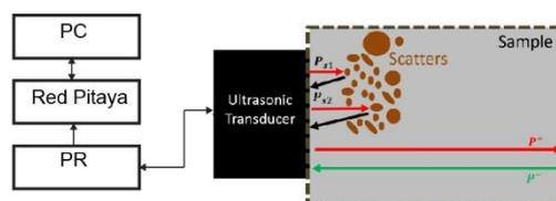
Figure 1. Experimental setup. The signal has been transmitted with the pulser-receiver, the received signals has been recorded with the red pitaya, and has been analyzed with MATLAB.
