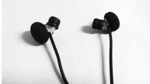
Figure 1. Binaural microphones used on the project.
