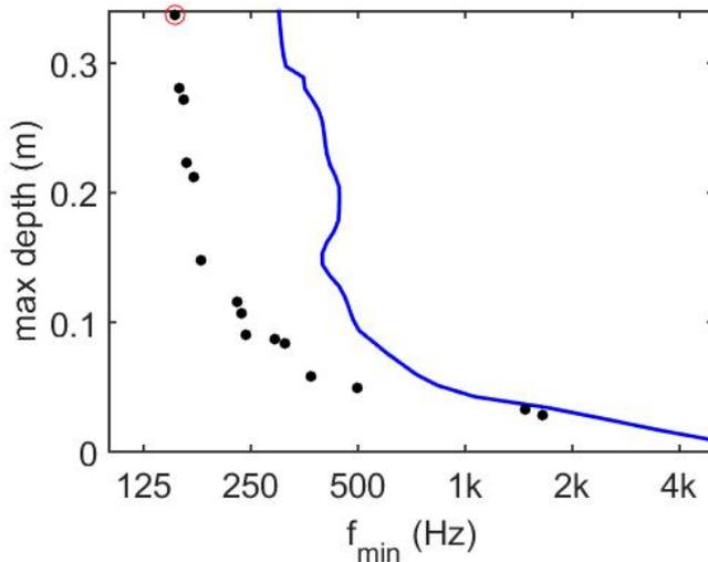
Figure 6.  $f_{min}$  for QR sound diffuser (width 1m) for different total depths (blue continuous line). Pareto front of the optimized diffusers (dots). The red circle correspond to the optimized diffuser illustrated in figure 7.
