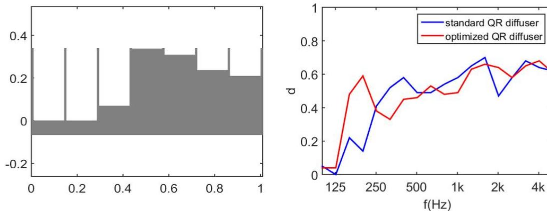
Figure 7. Left: Section of an optimized diffuser (red circle in figure 6). Right: Normalized diffusion coefficient versus frequency for a standard QR diffuser and the optimized diffuser illustrated on the left figure.
