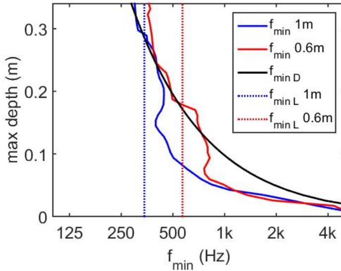
Figure 4.  $f_{min}$  for two different values of the width (1m (blue) and 0.6m (red)), Continuous lines . Theoretical  $f_{min}$  due to the limited depth of the diffuser (6), black line. Theoretical  $f_{min}$  due to the limited width of the diffusers (7), dotted lines.
