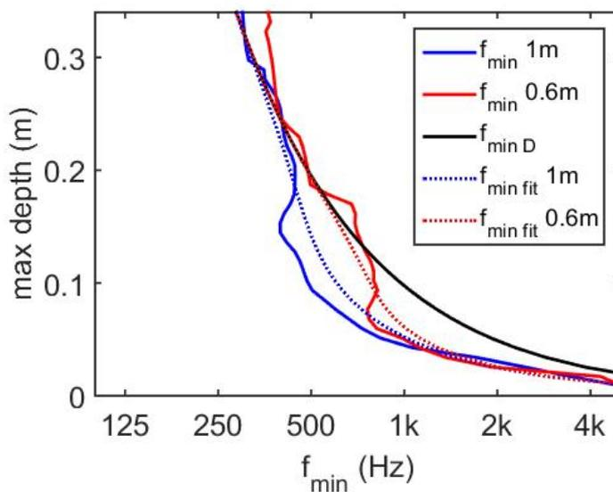
Figure 5.  $f_{min}$  for two different values of the width (1m (blue) and 0.6m (red)), Continuous lines . Theoretical  $f_{min}$  due to the limited depth of the diffuser (6), black line. Fits of  $f_{min}$  following equation (8), dotted lines.
