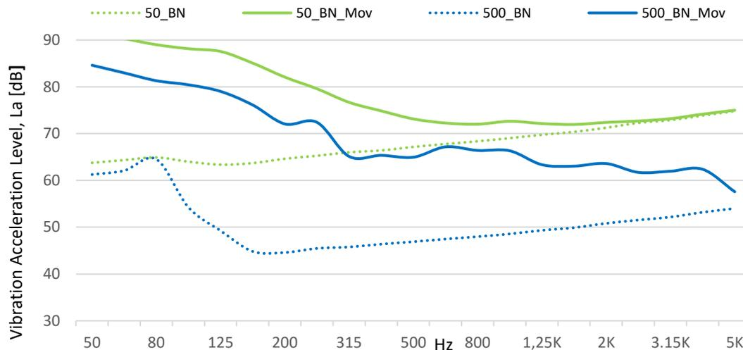
Figure 4. BN\_Mov experiment  $L_a$  and BN\_OnRubber (50\_BN and 500\_BN) experiment  $L_a$  comparison with 50mV/g and 500mV/g sensors.
