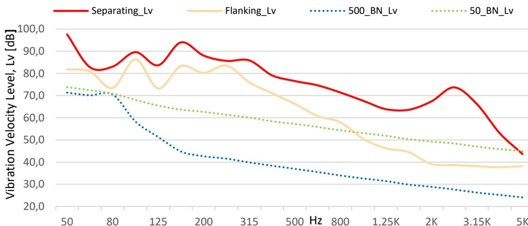
Figure 2. Separating element  $L_v$  and flanking element  $L_v$  comparison versus measurement system inherent noise  $L_v$  with 50mV/g and 500mV/g sensors performing BN\_OnRubber experiment.
