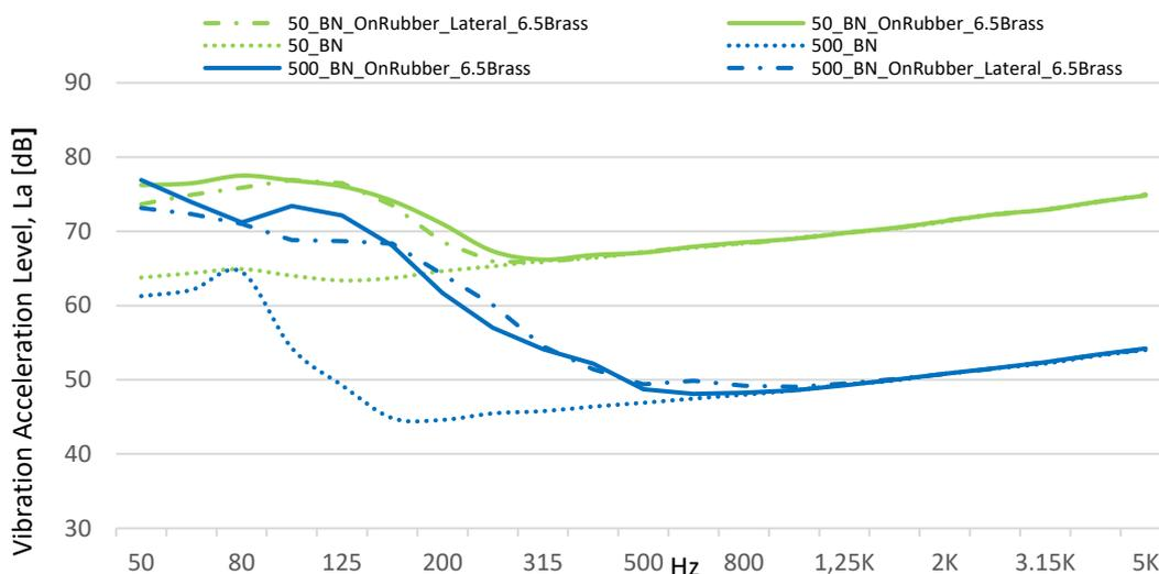
Figure 5. *BN\_OnRubber\_6.5Brass*  $L_a$ , *BN\_OnRubber\_6.5Brass\_Lateral* and *BN\_OnRubber* (*50\_BN* and *500\_BN*) experiment  $L_a$  comparison with 50mV/g and 500mV/g sensors.
