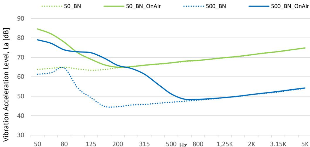
Figure 3. BN\_OnAir experiment  $L_a$  and BN\_OnRubber (50\_BN and 500\_BN) experiment  $L_a$  comparison, with 50mV/g and 500mV/g sensors.
