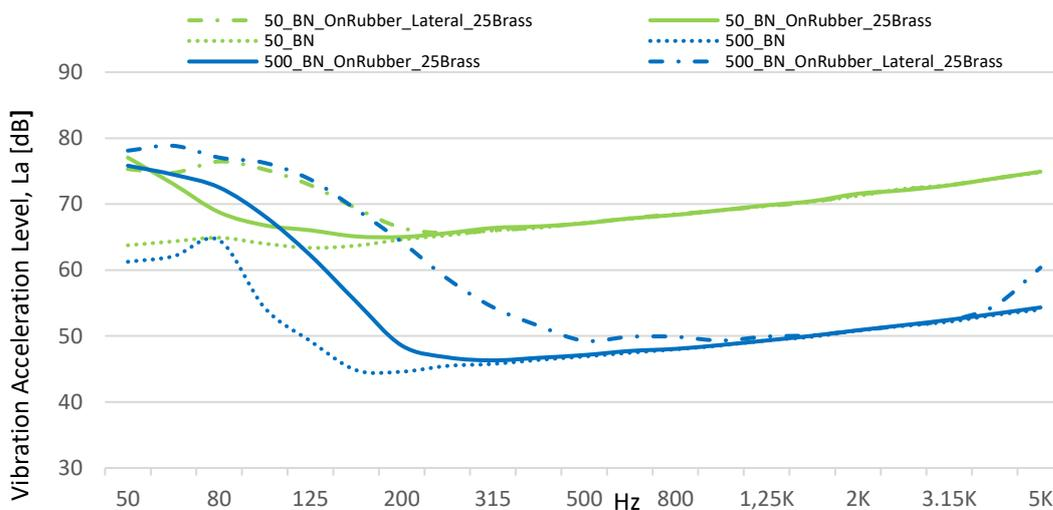
Figure 6. *BN\_OnRubber\_25Brass*  $L_a$ , *BN\_OnRubber\_25Brass\_Lateral* and *BN\_OnRubber* (*50\_BN* and *500\_BN*) experiment  $L_a$  comparison with 50mV/g and 500mV/g sensors.
