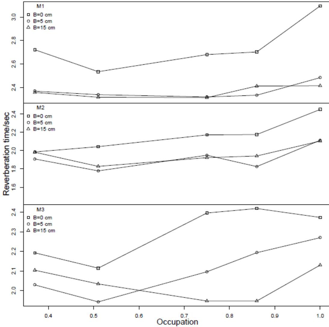
Figure 1: Reverberation time as a function of the occupation for the three different materials and the three levels of the air layer thickness, all of them for a fixed frequency of 800 Hz.
