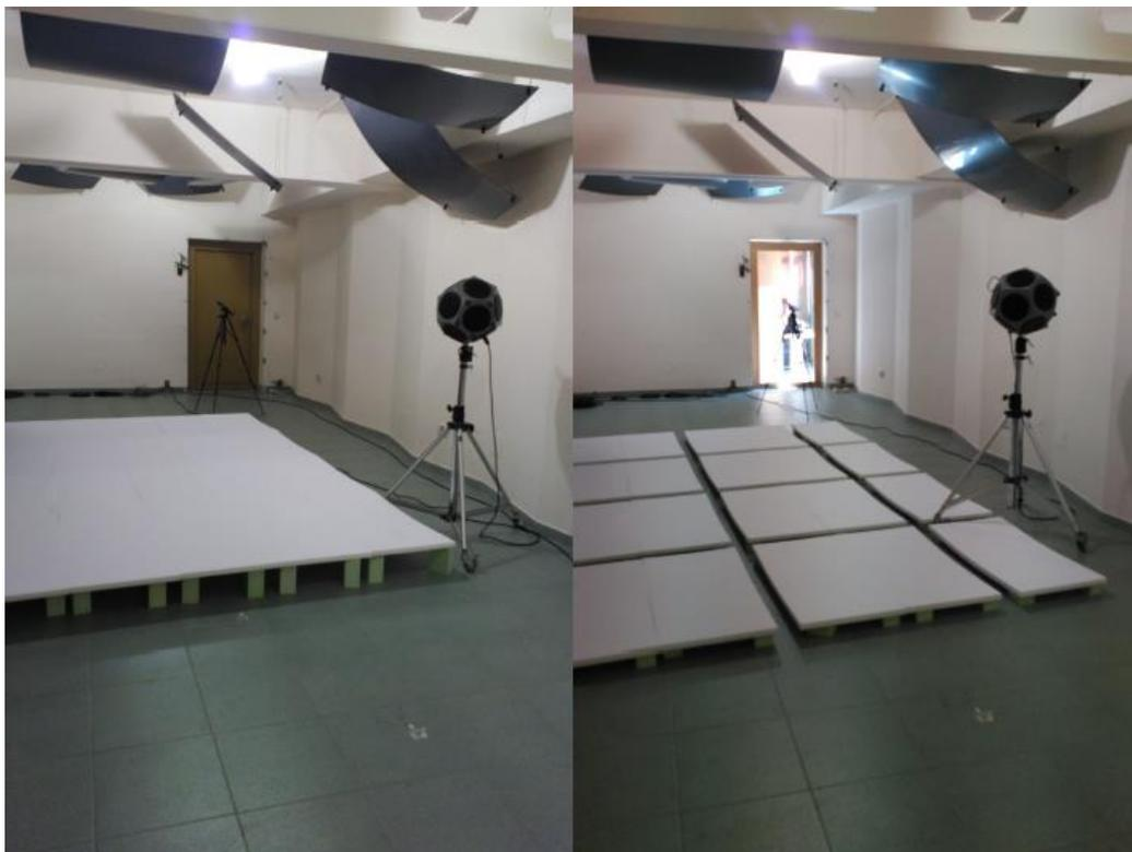
*Image 2: Two different arrangements of material M1: in the left side the material is laid in one piece (occupation 1) and with an air layer thickness of 15 cm; in the right side the material is laid in separated pieces, with an occupation of 0.86 and separated 5 cm from the floor.*
