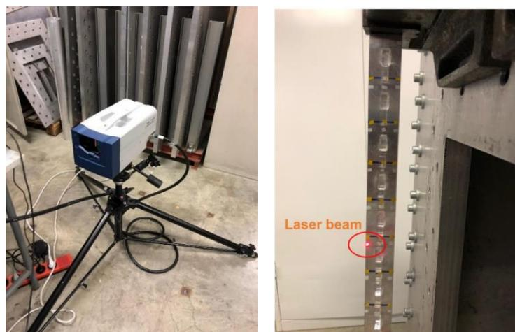
*Figure 14: (Left) Laser vibrometer (Right) Laser beam at a point to acquire the response in a metamaterial beam.*
