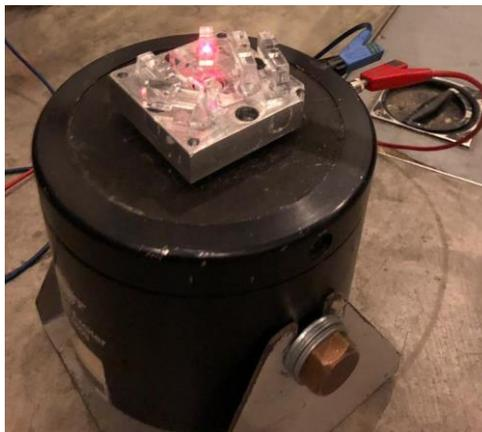
Figure 9: Test set up to retrieve the resonance frequency of the resonators.
