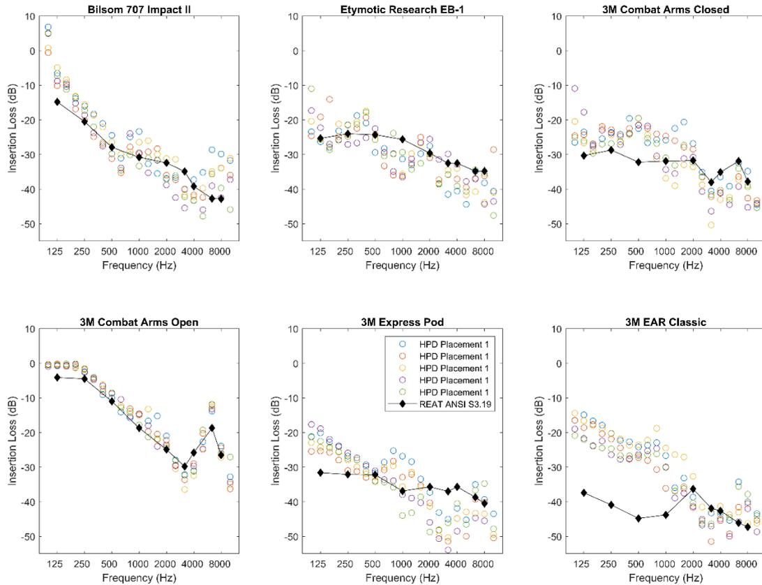
Figure 3. Comparison of ISIL results for each protector model and sample fitting with the Manufacturer's experimenter-fit REAT data.
