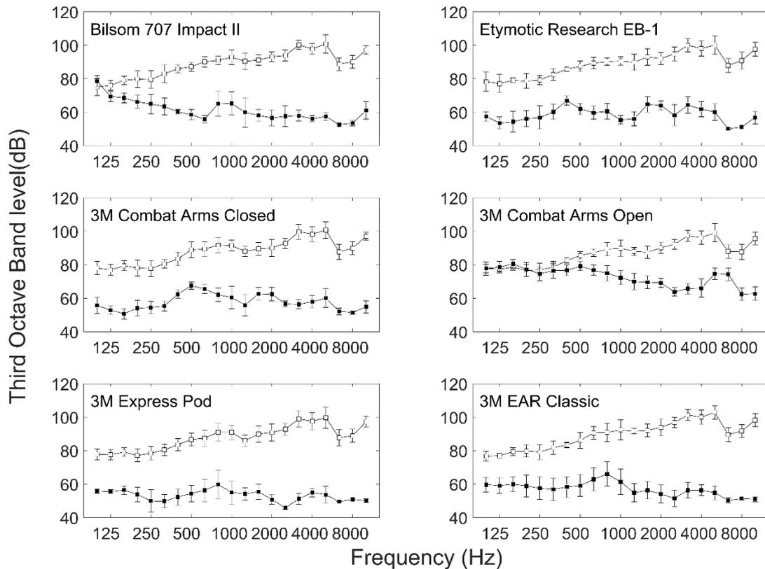
*Figure 2. The spectra of the unoccluded and occluded recordings of the ATF with different hearing protectors. The unoccluded levels are shown as open symbols. The occluded levels are shown as solid black symbols. The error bars represent one standard deviation.*
