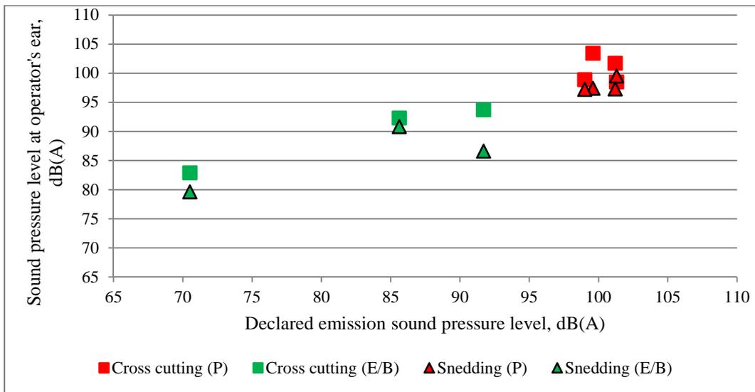
Figure 5: Declared emission  $L_{pA}$  plotted against simulated real use  $L_{pAeq}$  values during typical chain-saw operations. Note: P indicates data for petrol chain-saws; E/B indicates data for electric and battery operated chain-saws
