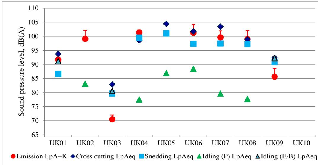
Figure 4: Comparison of declared emission  $L_{pA}$  and real use noise levels at the chain-saw operator's ear
