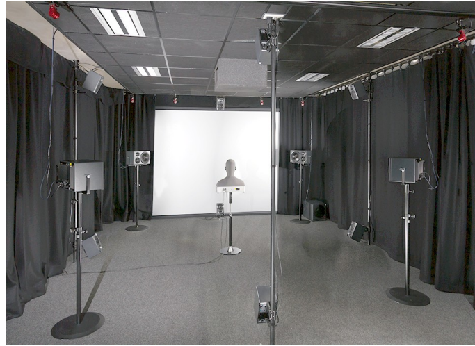
Figure 2: The figure shows the VRLab used to evaluate the proposed approach. The loudspeaker array is visible as well as the acoustics treatment in terms of curtains and an acoustic ceiling. The artificial head in the middle was used for measurements. During measurements the curtains covered the screen in front of the artificial head.
