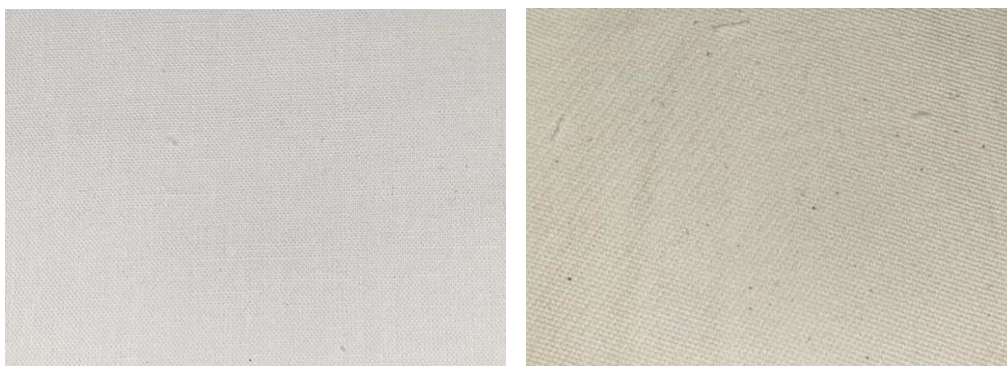
Figure 1. Textile fabrics used in this study. Left: CO fabric with a yarn density of 115 \text{ g/m}^2 ; Right: CO fabric with a yarn density of 210 \text{ g/m}^2 .
