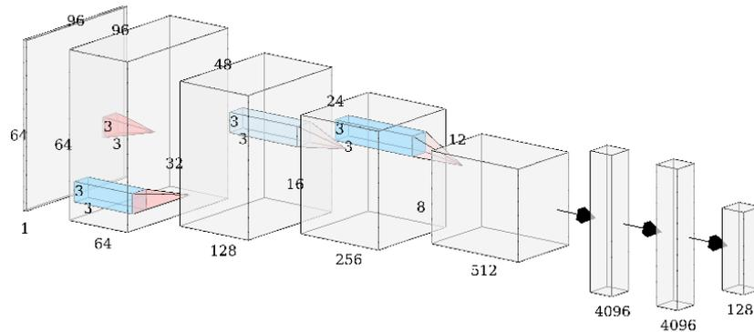
Figure 4. VGGish model architecture from Audioset (graph made using NN-SVG[7])
