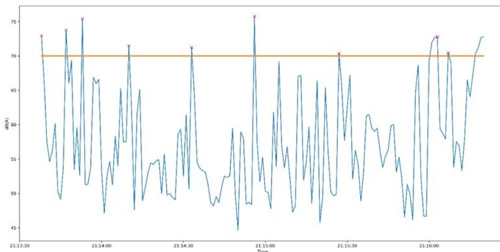
Figure. 5. Peaks detected on  $L_{Aeq,1s}$  data.
