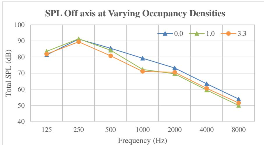
Figure 4 – Octave Band SPL – Off axis
