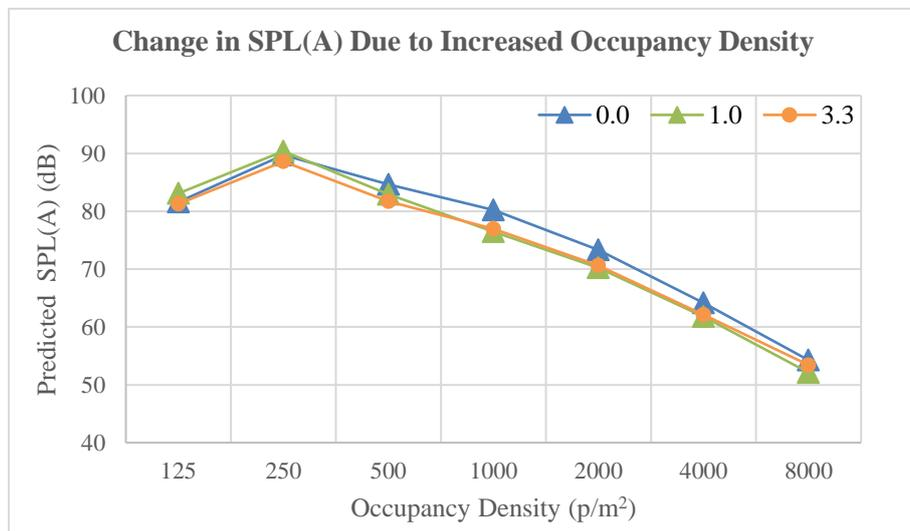
Figure 2 – Predicted SPL Under Varying Occupancy Densities
