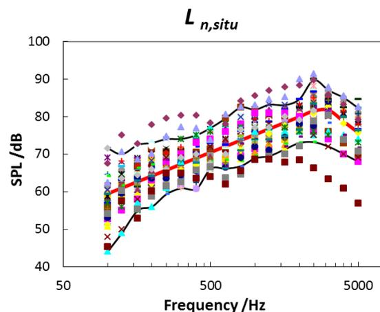
Figure 1 – Distribution of experimental data of impact sound pressure level measured for 40 bare floors in hollow-pots and concrete (in-situ).
