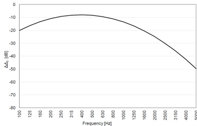
Figure 4 – Normalized correction spectrum  $\Delta\Delta_0$  to calculate contribution  $\Delta_0$  to be applied to  $\Delta L$  data measured on a concrete floor to estimate improved impact sound insulation on a CLT floor (values at 4000 Hz and 5000 Hz extrapolated from measured value up to 3150 Hz).
