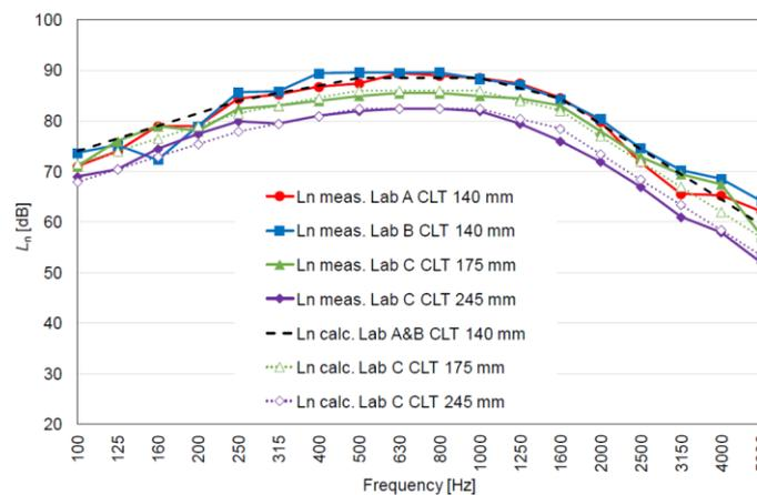
Figure 3 – Comparison between calculated reference floors ( $L_n$  calc) and laboratory measurements ( $L_n$  Lab) for bare CLT floors evaluated in Labs A, B and C.
