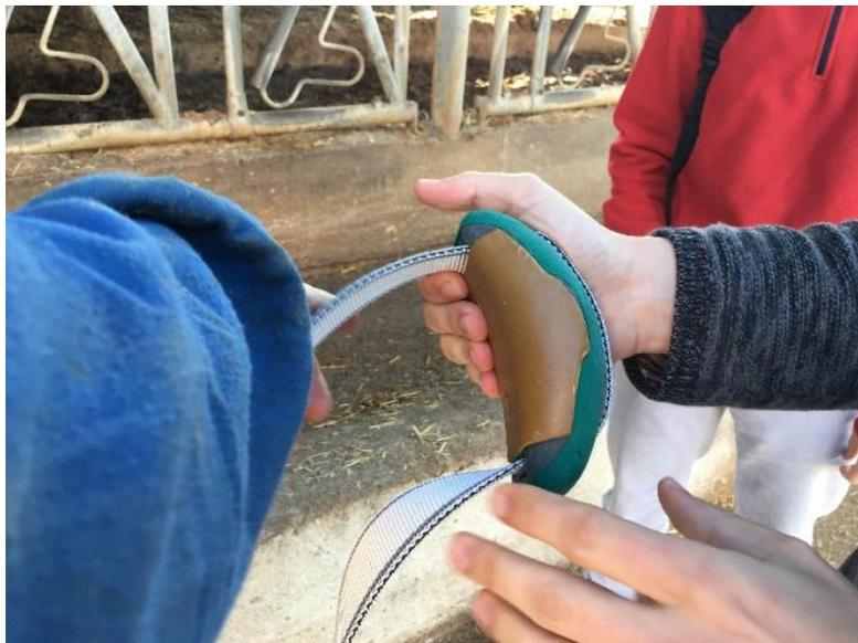
Figure 2: (left) The collar with the small recorder suspended inside, to record individual vocalizations during the drying-off, and (right), the installation of the acoustic sensor next to the calving cow beds.
