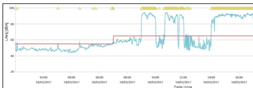
Figure 2 – Example of the temporal evolution of the sound immission level on a real-time platform.
