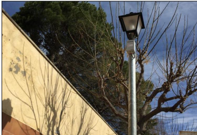
Figure 1 – View of one of the noise monitoring equipment installed in a streetlight.
