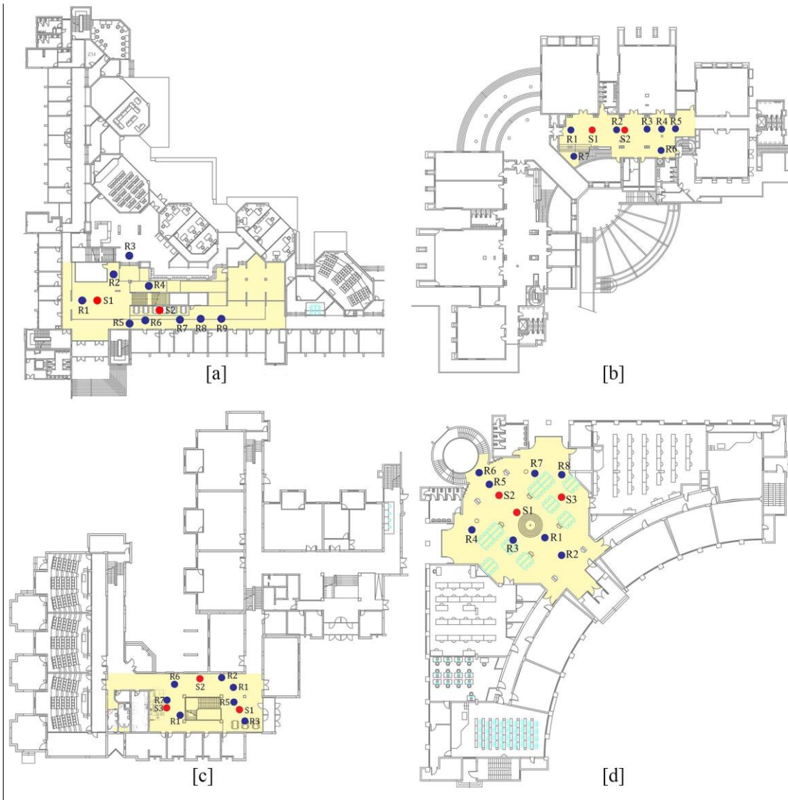
Figure 2 – Sources (S) and receivers (R) locations for each atrium in the field tests: a) A, b) FF, c) FC, d) SA building
