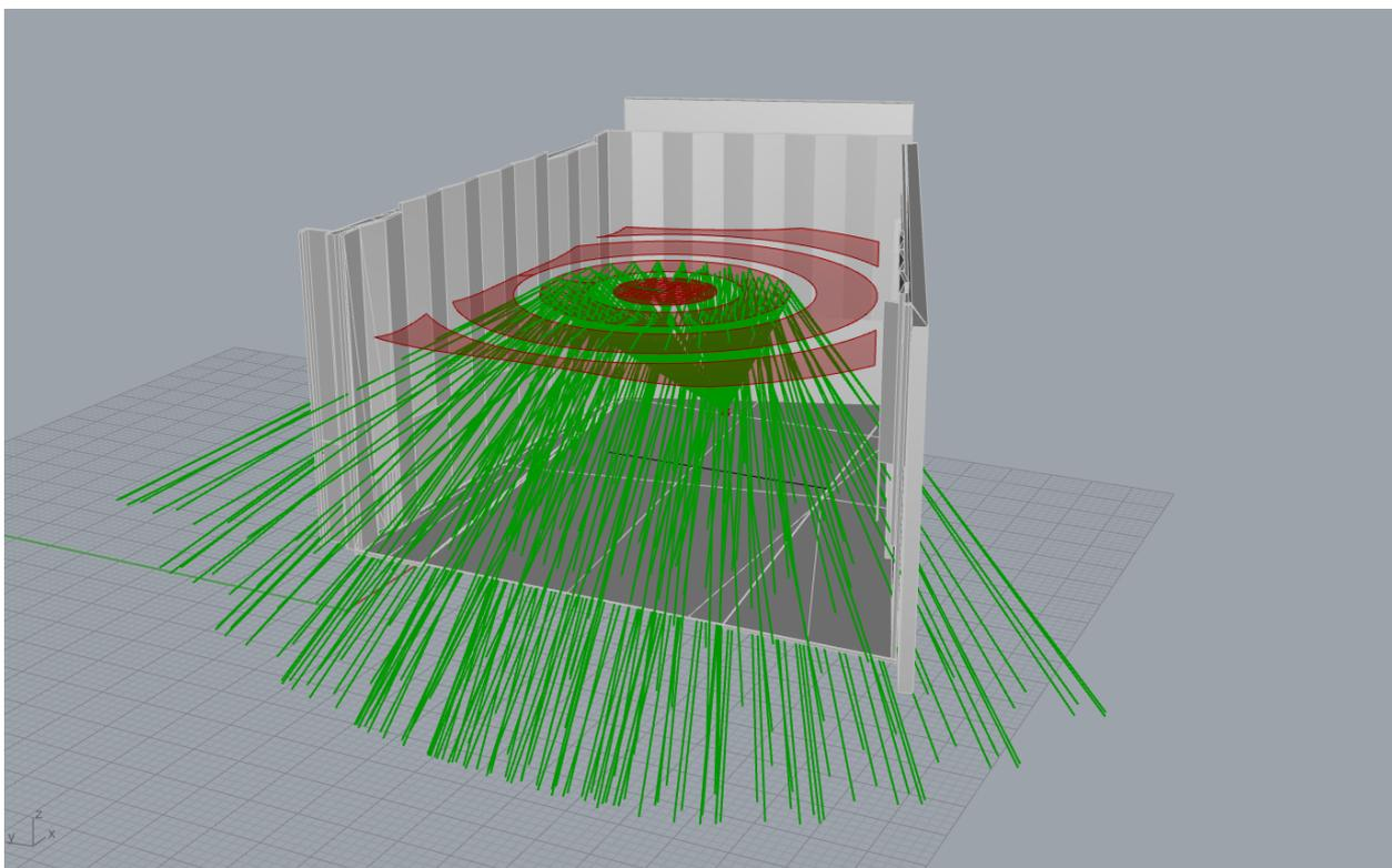
Figure 2 – First-order reflection distribution from a single ring element
