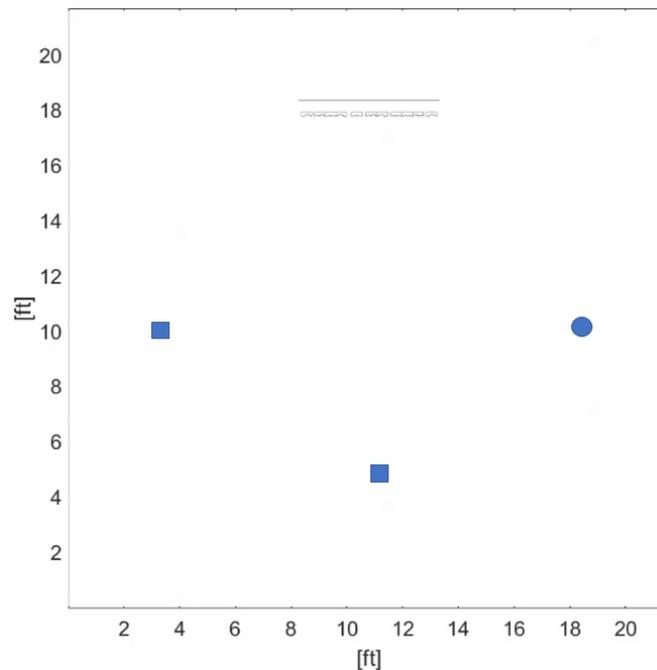
Figure 4 – Sample of the FDTD simulation setup. The circle depicts the location of the source and the squares depict receiver locations.
