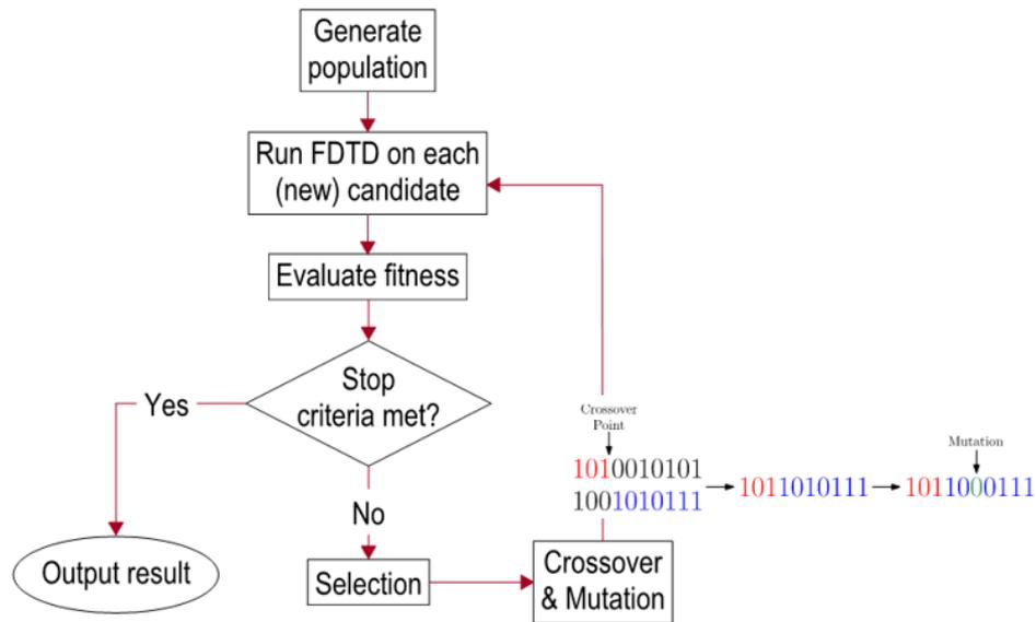
Figure 5 – Flow chart showing Genetic Algorithm process and crossover and mutation technique.
