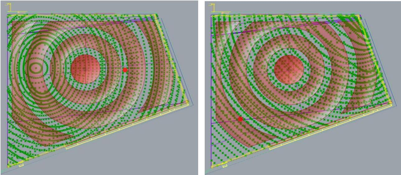
Figure 3 – First-order reflection hits on audience plane from entire array; ray source location in soloist position (left) compared to ray source location in far ensemble position (right)
