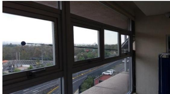
Figure 3 – Position of the microphone to measure the SPL of vehicular noise outside the classroom at 2 min front of the façade.
