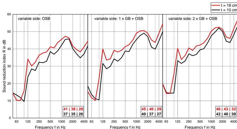
Figure 5: Influence of cavity thickness  $t = 10$  cm and  $t = 18$  cm, respectively at varied sheathing on one side of the single walls. The other side was always planked with 12 mm OSB. GB: gypsum board; SNQ  $R_w + C_{50-5000}$  |  $R_w + C_{tr,50-5000}$  in dB in the lower right corner of the graphs
