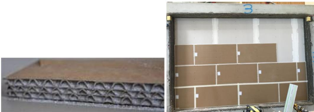
Figure 4: Left: sand board (corrugated cardboard filled with quartz sand, [www.wolf-bavaria.com](http://www.wolf-bavaria.com), 07/27/2021). Right: Application of sand boards on top of the gypsum boards. The sand boards were screwed into the studs.
