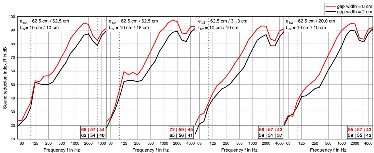
Figure 9: Influence of the gap width at the double wall and the interior OSB. Sheathings on exterior sides 2 x 12,5 mm GB and 12 mm OSB and on interior sides 12 mm OSB;  $e_{1/2}$ : distance between the stud centers at wall 1 and 2;  $t_{1/2}$ : cavity thickness at wall 1 and 2; SNQ  $R_w$  |  $R_w + C_{50-5000}$  |  $R_w + C_{tr,50-5000}$  in dB in the lower right corner of the graph
