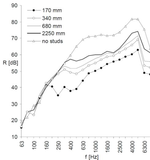
Figure 1: Influence of screw distance for lightweight, insulated test elements with metal sheathing and wooden studs [8]
