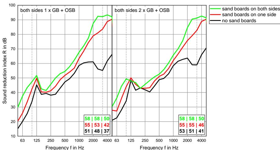
Figure 11: Influence of added GB and sand boards on a single wall with separated studs. SNQ  $R_w | R_w + C_{50-5000} | R_w + C_{tr,50-5000}$  in dB in the lower right corner of the graph
