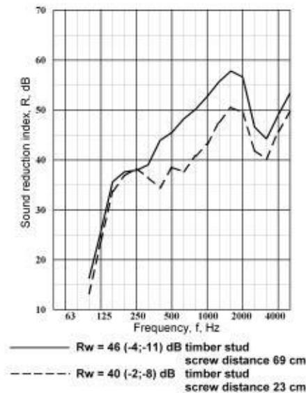
Figure 2: Influence of screw distance for insulated timber frame test element with gypsum board sheathing [9]
