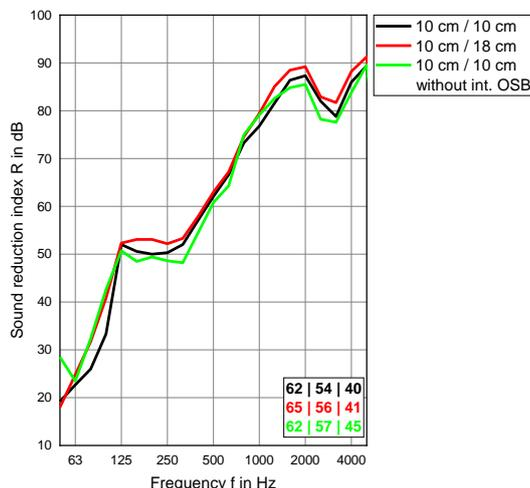
Figure 8: Influence of cavity thickness  $t_1 / t_2$  at the double walls and of an interior OSB (OSB at the gap); Sheathing on exterior sides 2 x 12,5 mm GB and 12 mm OSB and at interior side usually 12 mm OSB; SNQ  $R_w | R_w + C_{50-5000} | R_w + C_{tr,50-5000}$  in dB in the lower right corner of the graph
