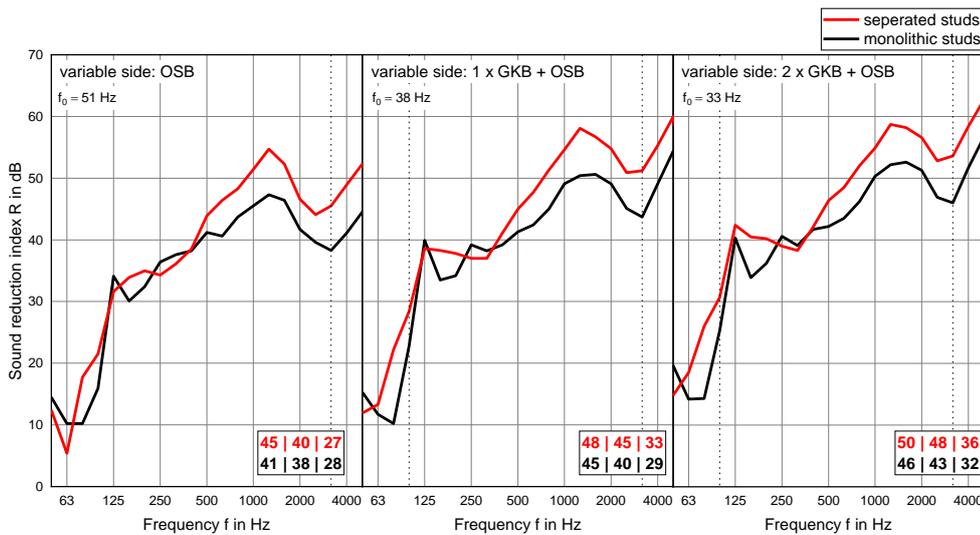
Figure 10: Influence of stud type in a single wall with variable sheathings at one side. Note that the frame is still continuous at the version with separated studs. Sheathing at the constant side 12 mm OSB; Cavity thickness = 18 cm;  $f_0$ : msm-resonance; SNQ  $R_w | R_w + C_{50-5000} | R_w + C_{tr,50-5000}$  in dB in the lower right corner of the graph
