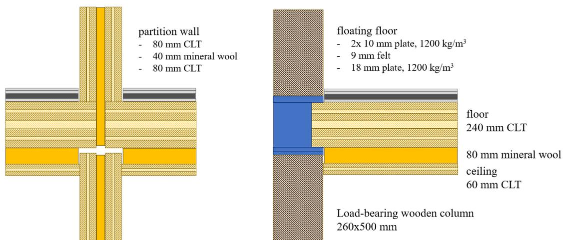
Figure 1. Wall, floor and ceiling constructions
