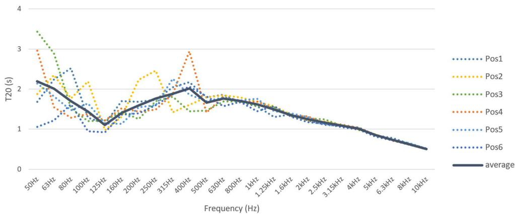
Figure 5. Reverberation time averaged from 6 source-receiver positions
