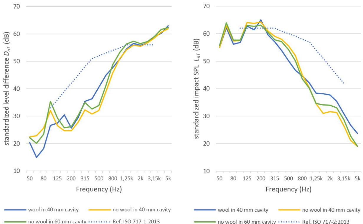
Figure 7. Measured airborne (left) and impact (right) sound insulation for the horizontal arrangement
