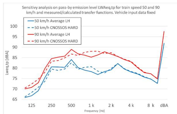
Figure 11. Comparison of calculated  $L_{WAeq,tp}$  spectra based on average measured Transfer Functions  $L_{HWR}$  and on CNOSSOS default data for hard monoblock track.
