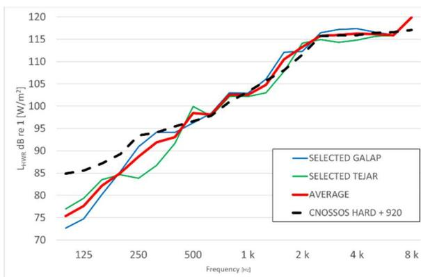
Figure 10. Average Total Transfer Function ( $L_{HWR}$ ) of both sites, compared to CNOSSOS input data for Total  $L_{HWR}$  for hard monoblock track and wheel diameter 920 mm (black dashed line).
