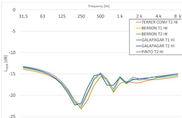
Figure 5-c: Transfer function  $L_{\text{HpW}}$  over the track (Excess attenuation) for high microphone positions
