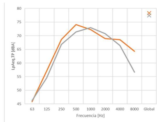
Figure 12-b. Comparison of A-weighted pass-by sound levels, measured (grey line) and calculated (orange line) at 94 km/h, Galapagar site.
