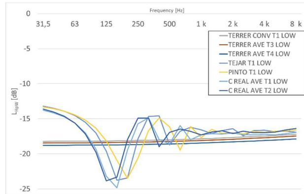
Figure 5-b: Transfer function  $L_{\text{HpW}}$  over the ground (Excess attenuation) for low microphone positions
