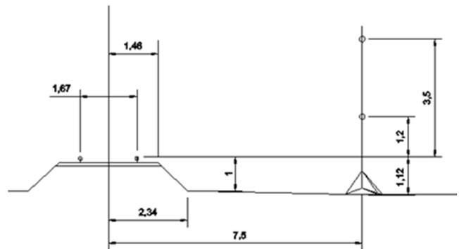
Figure 4: Measurement and site geometry for single track conventional line at El Tejar. Near Track as in fig 2b mT2lo and mT2hi.
