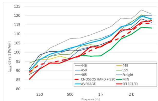
Figure 9-a. Total Transfer Function ( $L_{HWR}$ ) at the Tejar site per train type, compared to CNOSSOS input data for hard monoblock track (red dashed line)
