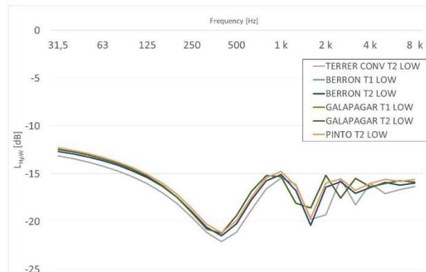
Figure 5-d: Transfer function  $L_{\text{HpW}}$  over the track (Excess attenuation) for low microphone positions
