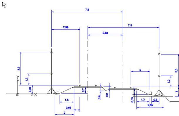
Figure 3: Measurement and site geometry for conventional line at Galapagar (as in fig 2a)
