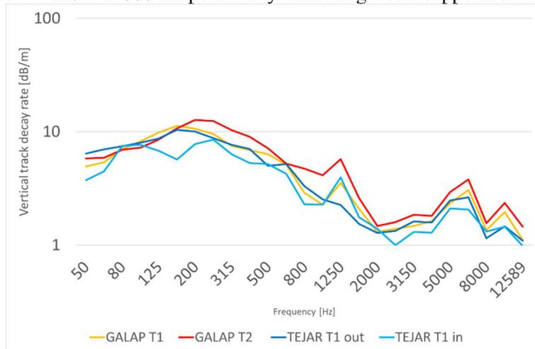
Figure 8: Spectrum of vertical track decay rates in [dB/m] in third octave bands for the Galapagar and Tejar sites, derived from pass-by rail acceleration time signals.
