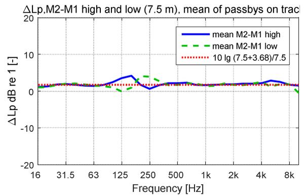
Figure 7: average difference between over track and near track microphones for high and low positions, and calculated with 10 lg d distance free field correction. Series of pass-bys on track 2 at Pinto site.
