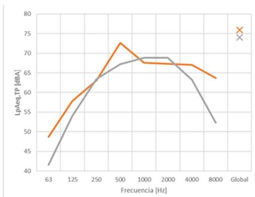
Figure 12-a. Comparison of A-weighted pass-by sound levels, measured (grey line) and calculated (orange line) at 75 km/h, Tejar site.
