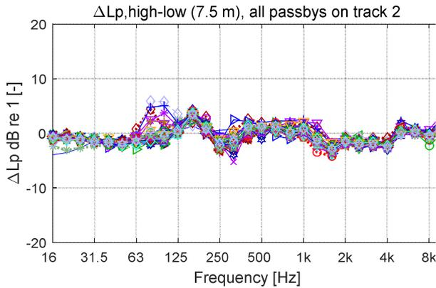
Figure 6. Difference between high and low microphone for several pass-bys on one track at Pinto site
