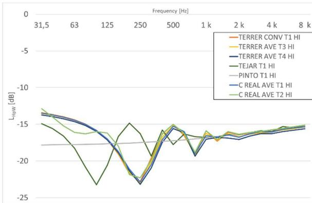
Figure 5-a: Transfer function  $L_{\text{HpW}}$  over the ground (Excess attenuation) for high microphone positions
