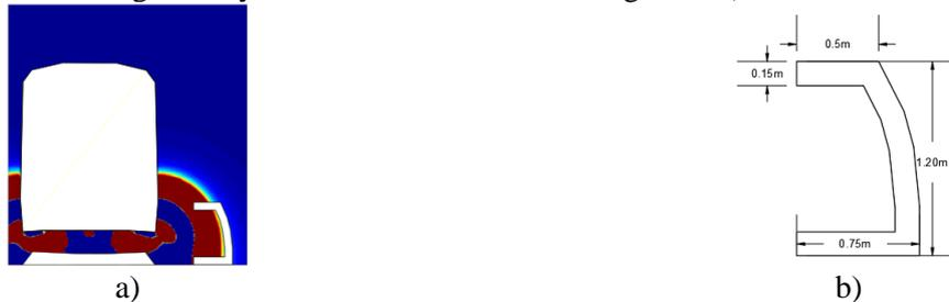
Figure 7 - (a) Schematic representation of the wave front and the designed barrier; (b) Representation of the main dimensions of the final barrier.
