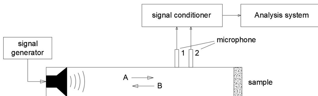
Figure 3. Experimental set-up used to obtain the acoustic impedance of the masks
