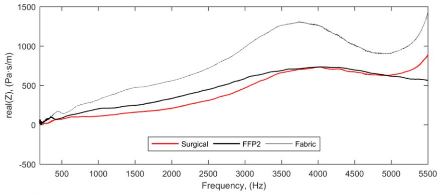
Figure 5. Real part of the acoustic impedance for different masks.
