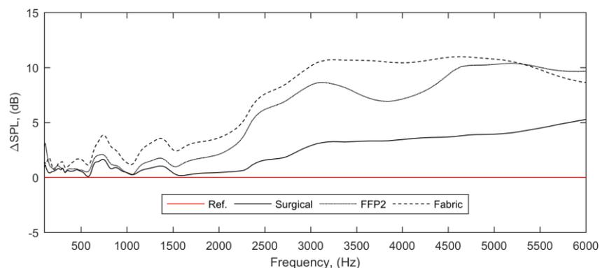
Figure 4. Attenuation level obtained for the different masks. Reference corresponding to situation without mask.
