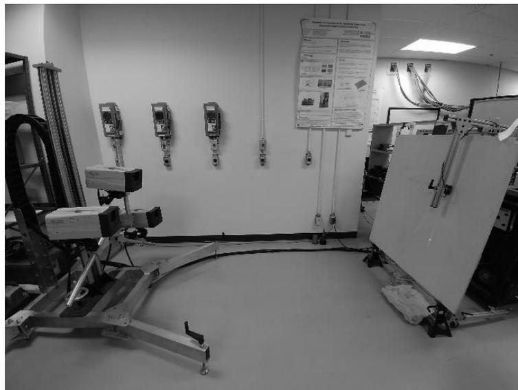
Figure 1 - Measurement setup for the determination of the dispersion relations in plywood. Panorama of the panel and the laser Doppler vibrometer, with detail of the clamping of the panel and detail of the fixing of the piezo.
