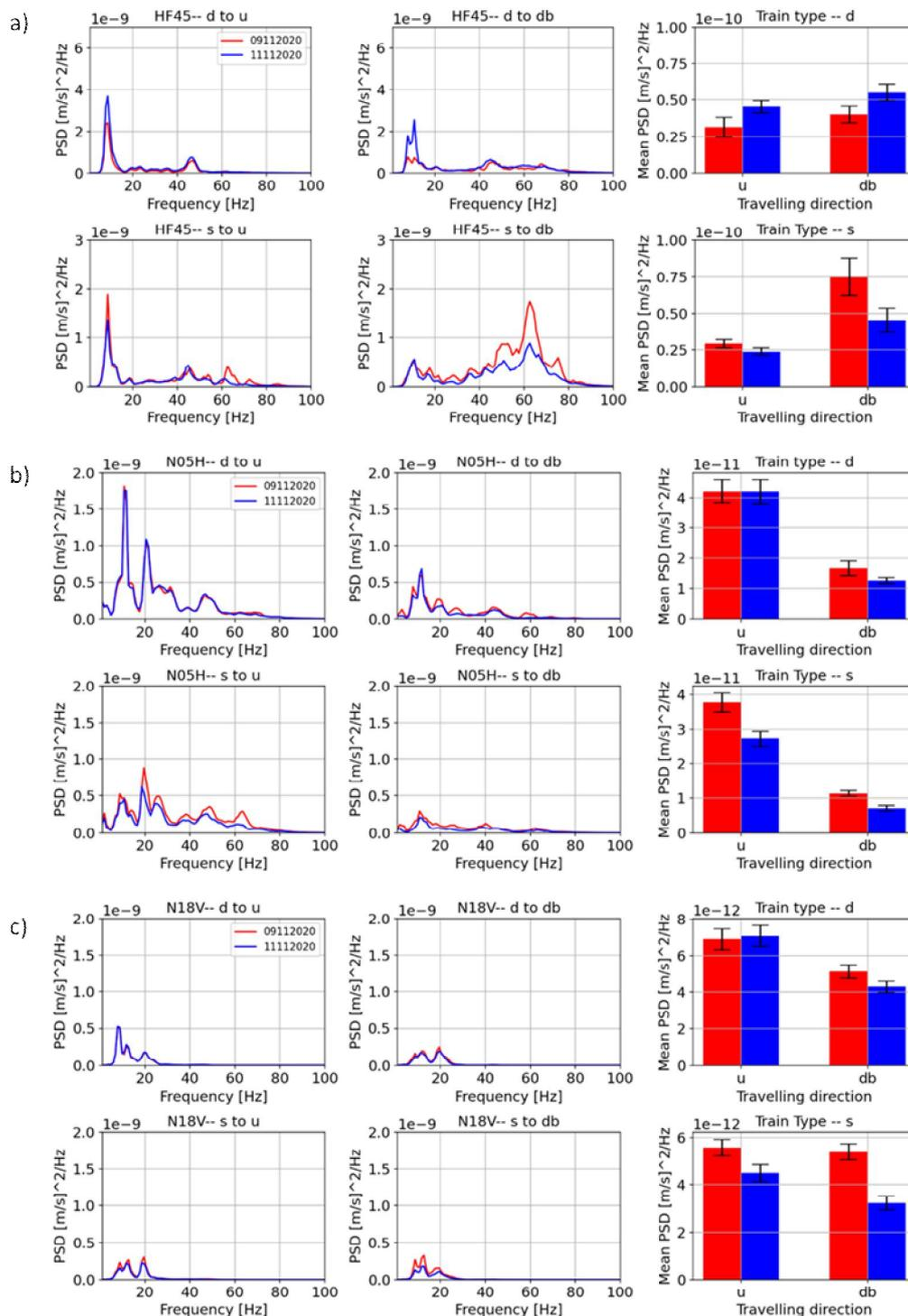
Figure 9 Comparison of the results in a) HF geophone in embankment, b) vertical vibration at 5 m from eastern track (9 m from western track) and c) vertical vibration at 18 m from eastern track (23 m from western track)
