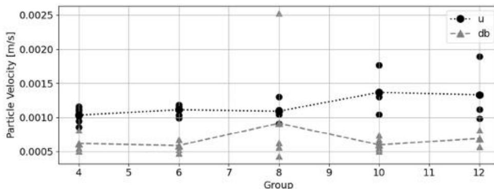
Figure 3 Vibration velocity  $V_{max}$  of train pass-by's at 5 m (northbound  $\bullet\bullet\bullet$  u) and 9m (southbound  $\triangle\triangle\triangle$  db) as a function of train length ((number of carriages per train) for train type VIRM double decker
