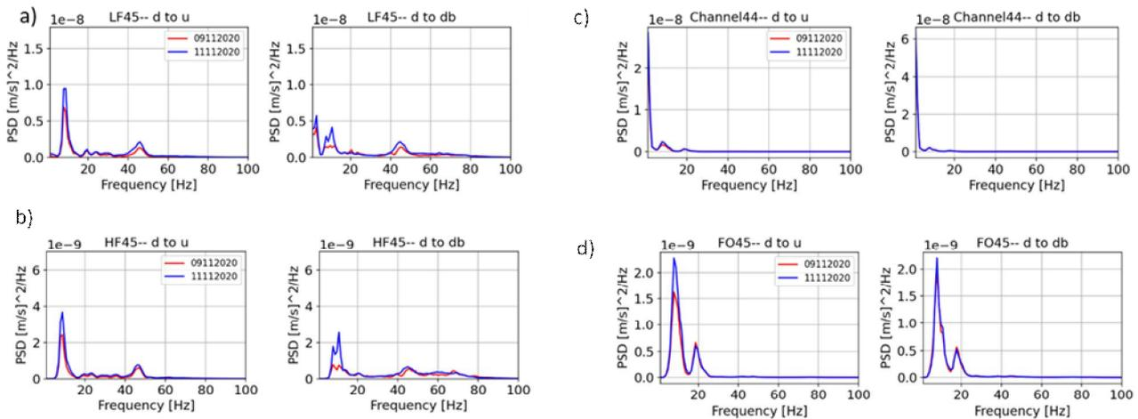
Figure 8 PSD from measurements at position 45 m on embankment. a) 1 Hz geophone, b) 4.5 Hz geophone, c) fibre optics filtered at 1 Hz (low cut) and d) fibre optics filtered at 4.5 Hz (low cut). It refers to double deckers, in both directions (to u is to Utrecht (northbound) and to db is to Den Bosch (southbound)).
