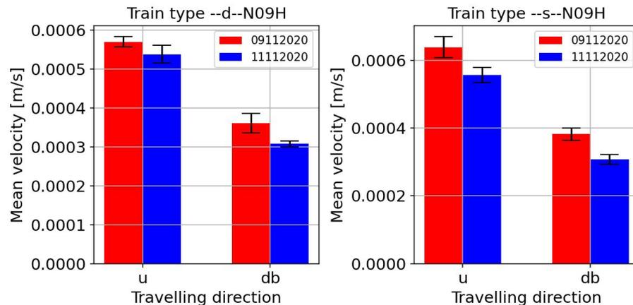
Figure 5 Comparison of maximum velocity for horizontal vibrations over all train pass-by's before (red) and after (blue) maintenance works at signal N09H. See text for more information.
