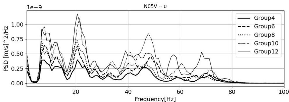
Figure 4 Power spectral density for vertical vibrations in point N05 for passing double decker, influence of train composition (group is number of wagons).
