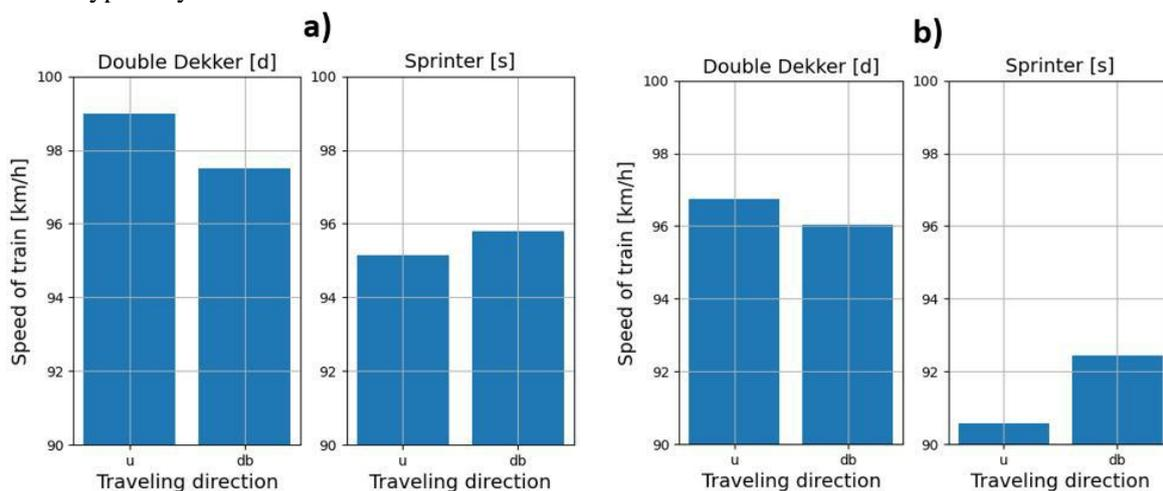
Figure 2 Average train speed during measurements a) at 9 November and b) at 11 November. u means direction Utrecht (Northbound) and db means direction den Bosch (Southbound)
