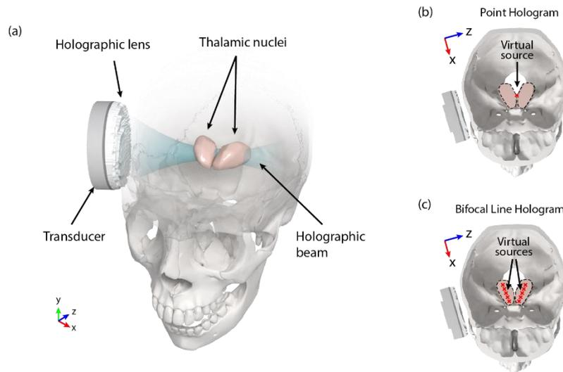
Figure 1: a) Scheme of the transtemporal transducer-lens system for thalamic focusing. b) point hologram virtual source location. c) Bifocal line hologram virtual sources location.
