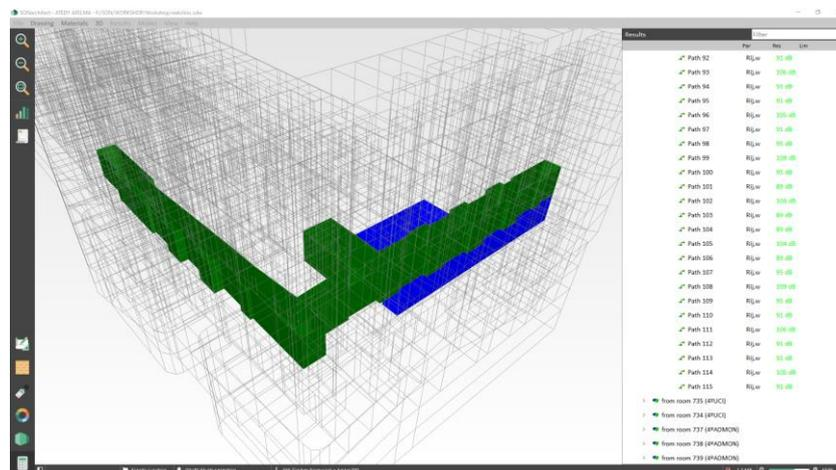
Figure 5 - 3D view of a compliant pair of rooms and the list of transmission paths (115)
