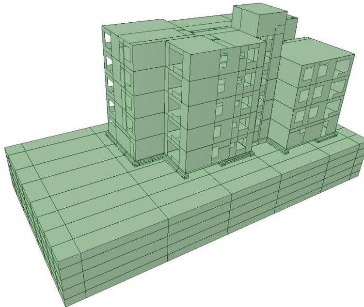
Figure 2 – Numerical model of the building.
