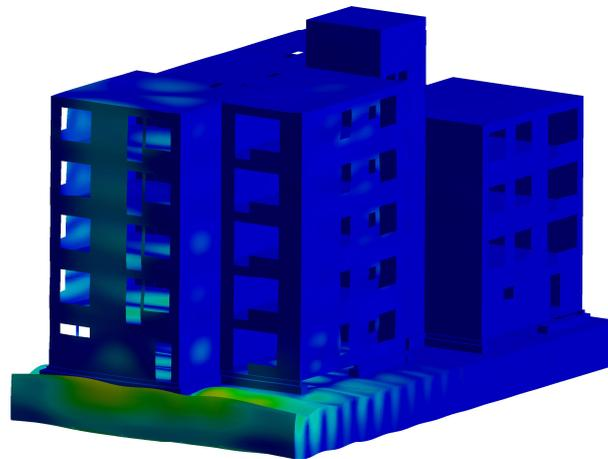
Figure 4 – Visualization of vibration in the numerical model. PML regions and parts of the modelled ground are not shown.
