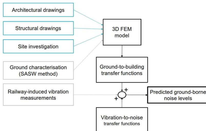
Figure 3 – Block diagram of the proposed evaluation method.
