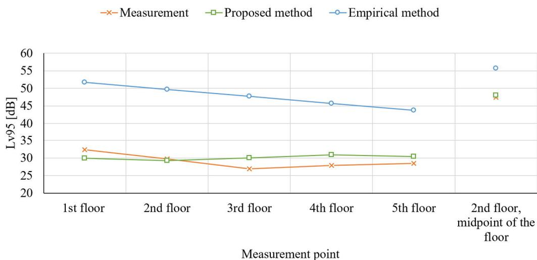
Figure 5 – Comparison of evaluation methods and measurements in the building.
