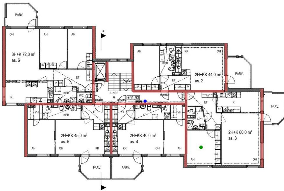
Figure 1 – The floor plan of the investigated building. The walls marked with red are load bearing. Also shown are the measurement points in the load bearing structures (blue dot), midpoint of the floor (green dot) and ground (red dot).
