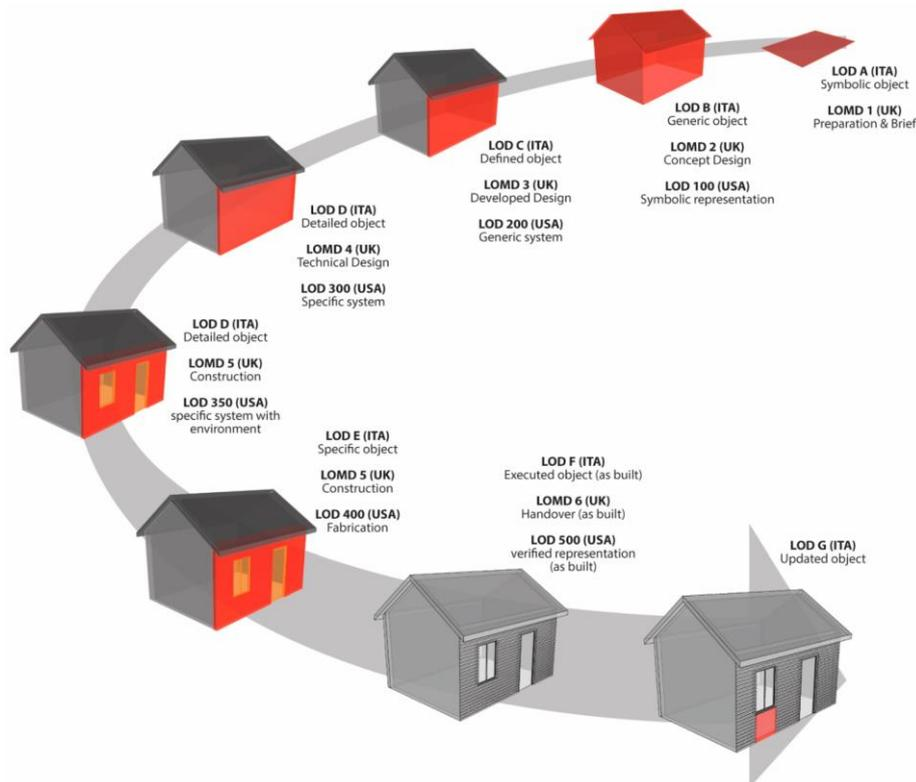
Figure 2 – Level of detail (LoD)’s progression according different national references with relative comparison [18].
