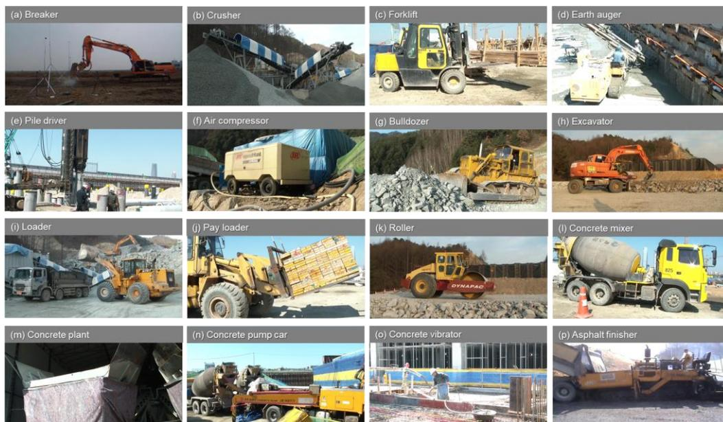
Figure 1 – Photos of sixteen construction machines.
