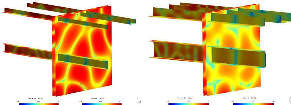
Figure 4 – Bedrooms: incident pressure (dynamic range 60 dB) and normal velocity (dynamic range 180 dB) (resp. source and receiver volumes). Left) 30 cm square posts, right) 60 cm square post. 500 Hz.
