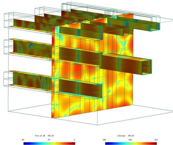
Figure 3 – Global view in the case of large volumes (living rooms) at 500 Hz. Source volume (left): incident pressure. Receiver volume (right): normal velocity.
