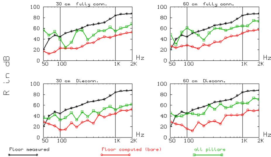
Figure 8 – Transmission Loss R in dB for the large volumes. Two post sizes, two types of floor/posts contact.
