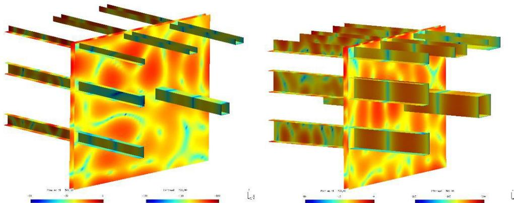
Figure 7 – Living rooms: incident pressure (dynamic range 60 dB) and normal velocity (dynamic range 180 dB) (resp. source and receiver volumes). Left) 30 cm square posts, right) 60 cm square post. 500 Hz.
