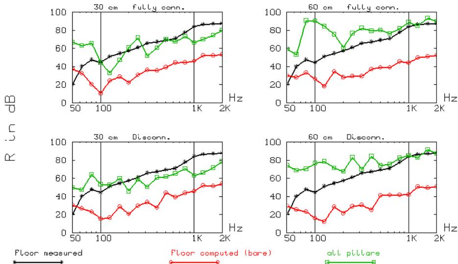
Figure 5 - Transmission Loss R in dB for the small volumes. Two post sizes, two types of floor/posts contact.
