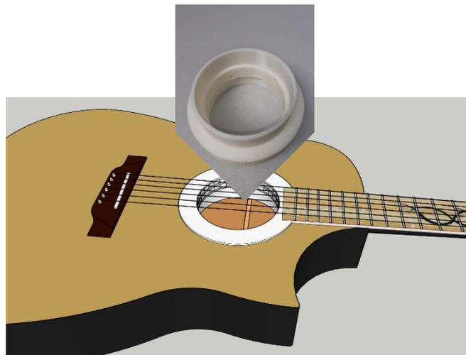
Figure 1: The tunable resonator described in this study, applied to an acoustic guitar sound hole.
