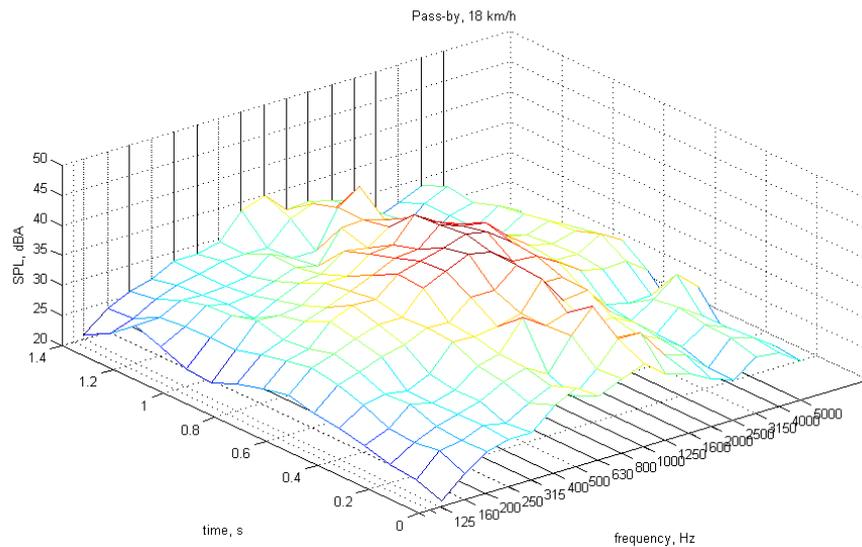
Figure 3. Spectrogram of tested HEV at 18 km/h
