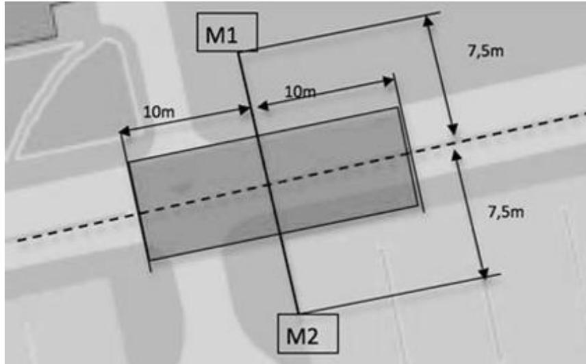
Figure 1. Pass-by test configuration for sound samples acquisition.
