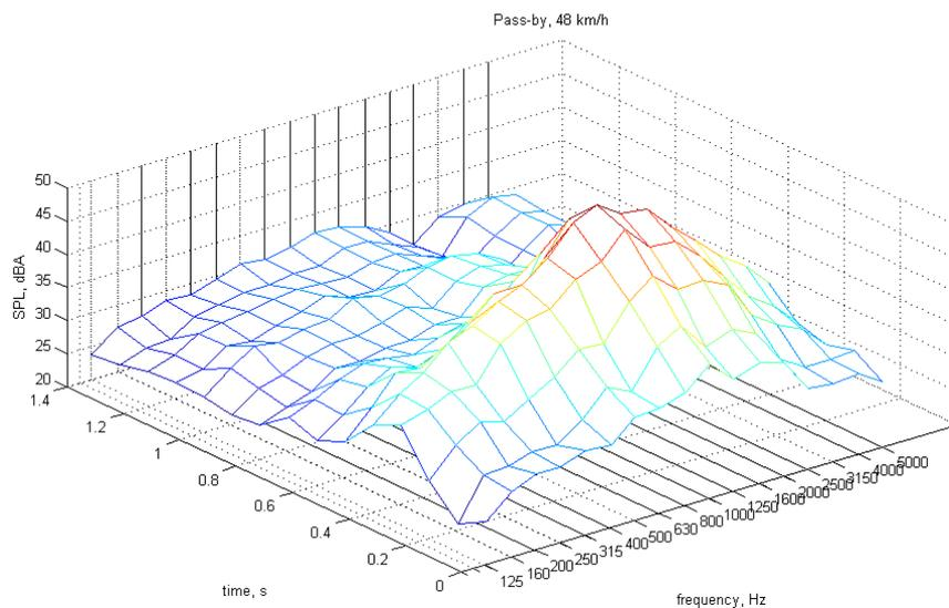
Figure 5. Spectrogram of tested HEV at 48 km/h
