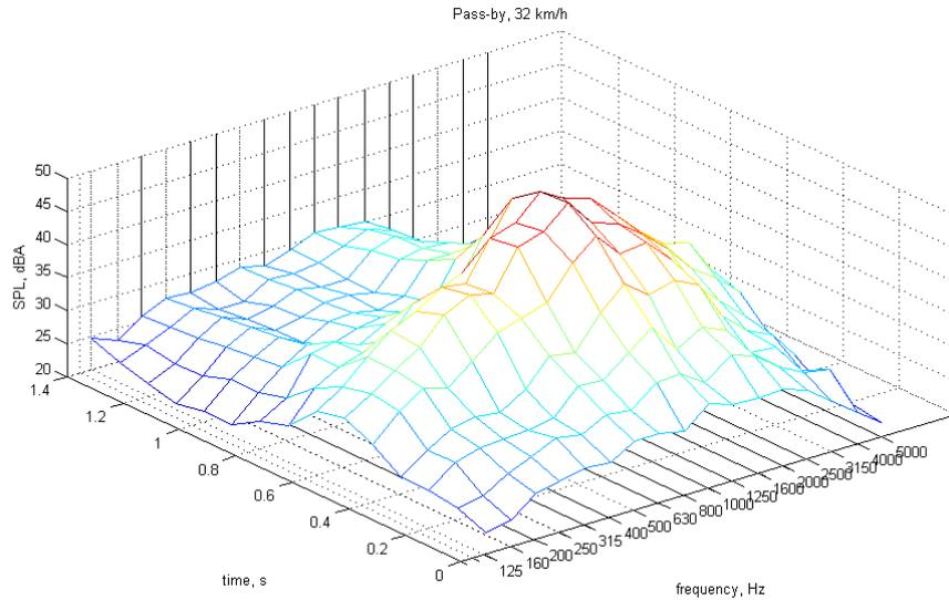
Figure 4. Spectrogram of tested HEV at 32 km/h
